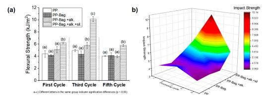
**Figure 3.** (a) Impact properties of PP and PP-Bagasse biocomposites and (b) 3D colormap surface of the impact properties.
