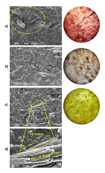
**Figure 17.** SEM (**left**) and optical micrographs (**right**) for 5th processing cycle: (**a**) PP.Bag., (**b**) PP-Bag + Alk. and PP-Bag + Alk. +sil. (**c**,**d**).
