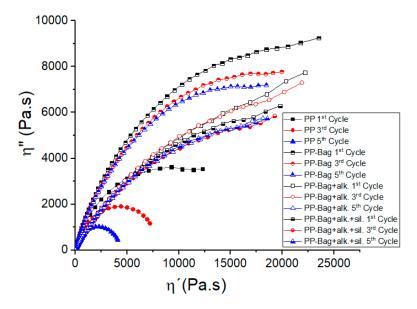
Figure 12. Cole–Cole plots of PP and PP-Bagasse biocomposites.
