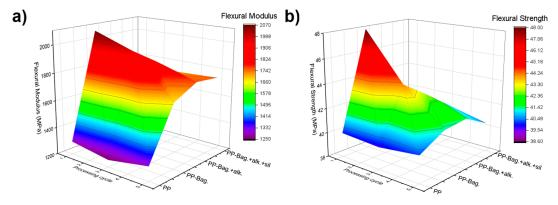
**Figure 2.** Three-dimensional colormap surface of flexural modulus (**a**) and flexural strength (**b**) of PP and PP-Bagasse biocomposites.
