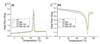
**Figure 5.** (a) Cooling and (b) second heating DSC curves for third processing cycle PP and PP-Bagasse biocomposites.
