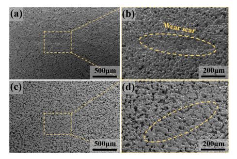
**Figure 9.** The SEM image of wear scar under dry friction, and (b) wear scar diagram in the yellow circle of (a) at higher magnification; (c) the SEM image of wear scar under oil lubrication conditions, and (d) wear scar diagram in the yellow circle of (c) at higher magnification.
