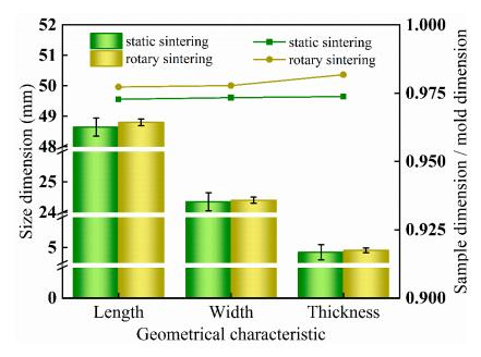
Figure 2. Dimension of samples obtained under the two different molding conditions.
