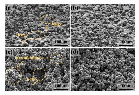
**Figure 4.** Microstructure of the sample under different forming states: (a,b) Surface microstructure of the sample under the molding condition of static sintering and rotary sintering, respectively. Arrows in (c) indicate the bulges and dents in the surface; (c,d) cross-sectional microstructure of sample under the molding condition of static sintering and rotary sintering. Arrows in (c) indicate the closely packed and large holes of the porous microstructure.
