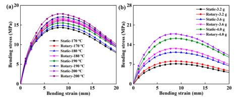
**Figure 7.** The bending strength of the product under different process conditions: (a) Trends of bending behavior of samples obtained by different molding methods with respect to the change in temperature when the charging amount was 4 g, and (b) trends of bending behavior of samples obtained by different molding methods with respect to the change in charging amount when the sintering temperature was 200 °C.
