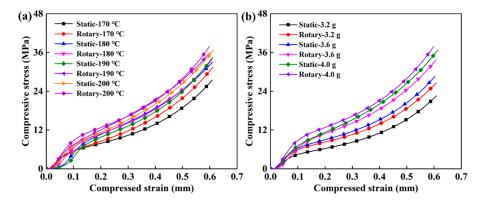
**Figure 6.** The compressive strength of the sample under different process conditions: (a) Trends of compression properties of samples obtained by different molding methods with respect to the change in temperature when the charging amount was 4 g, and (b) trends of compression properties of samples obtained by different molding methods with respect to the change in charging amount when the sintering temperate was 200 °C.
