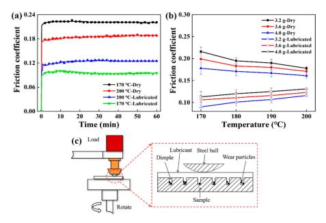
**Figure 8.** The friction and wear performance comparison of the samples: (a) The friction curve of the sample under different porosity and working conditions when the charging amount was 3.2 g, (b) coefficient of friction of samples under different porosity and working conditions, and (c) schematic diagram of friction and wear under different working conditions.
