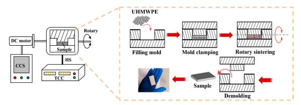
**Figure 1.** Schematic diagrams of the dynamic rotary sintering device and the fabrication procedure of the ultra-high-molecular-weight polyethylene (UHMWPE) porous materials using the device.
