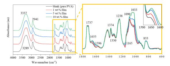
Figure 5. Fourier Transform Infrared (FTIR) spectra of pure PVA and hemp/PVA composite films.
