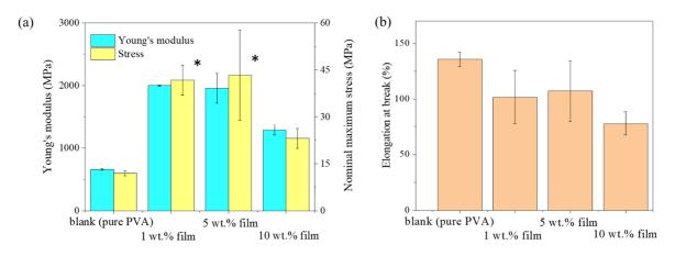
**Figure 6.** Mechanical properties of pure PVA and hemp/PVA composite films: (**a**) Young's modulus and nominal maximum stress (**b**) Elongation at break (%). \* denotes significant difference ( $p \le 0.05$ ) was found between data.
