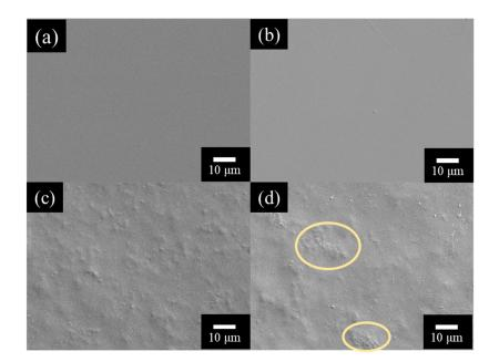
**Figure 3.** The surface of hemp/PVA composite films with different hemp particle weight ratios (**a**) 0%, (**b**) 1%, (**c**) 5%, (**d**) 10%.
