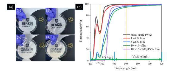
**Figure 8.** (a) Photographs of the film: (1) pure PVA, (2) 1 wt. % film, (3) 5 wt. % film, (4)10 wt. % film; (b) Transmission spectra of the composite films with various hemp hurd additions in this study and TiO<sub>2</sub>/PVA film reproduced from Liu et al. [42].
