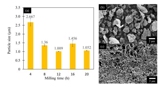
**Figure 1.** (**a**) Particle size as a function of wet milling time; scanning electron microscope (SEM) images of hemp particles: (**b**) after 4 h and (**c**) after 20 h of wet ball-milling.
