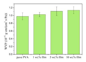
Figure 7. Water vapor permeability (WVP) of hemp/PVA composite films versus hemp loadings.
