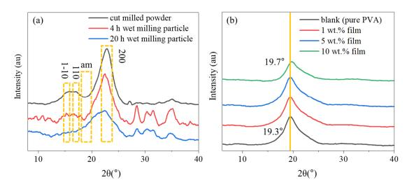
Figure 2. X-ray diffraction (XRD) pattern of (a) hemp particles and (b) composite films.
