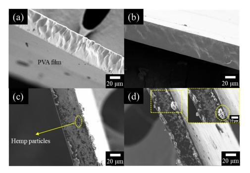
**Figure 4.** The cross-section images of hemp/ polyvinyl alcohol (PVA) composite films with different hemp particle weight ratios: (**a**) 0%, (**b**) 1%, (**c**) 5%, (**d**) 10%.
