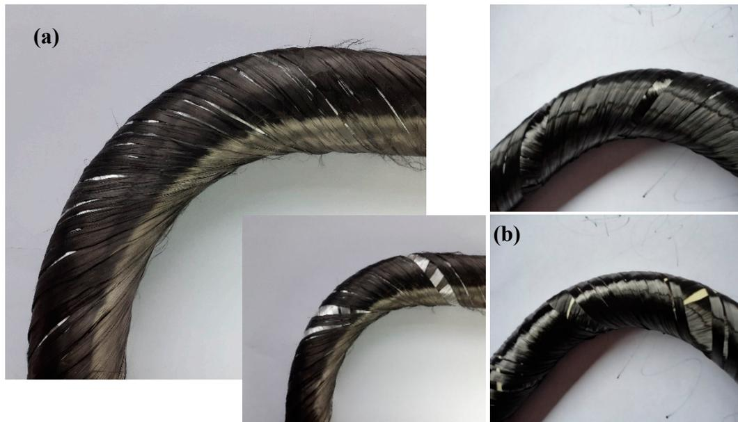
**Figure 14.** Image of the polymer composite frames wound using (a) the new and (b) manual-robot winding processes.
