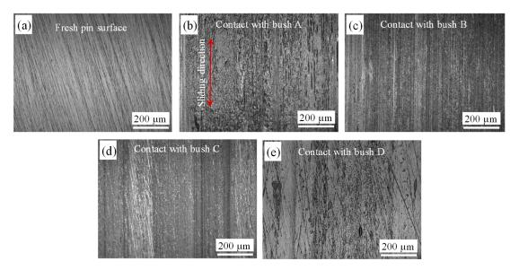
**Figure 9.** Microscopic images of the shaft surfaces, (**a**) fresh surface; (**b**) contacted with Bush A; (**c**) contacted with Bush B; (**d**) contacted with Bush C; (**e**) contacted with Bush D.
