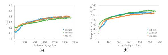
**Figure 3.** Three repeat wear tests for Bush A: (**a**) CoF varying with articulating cycles; (**b**) temperature rise in the bush wall varying with articulating cycles.
