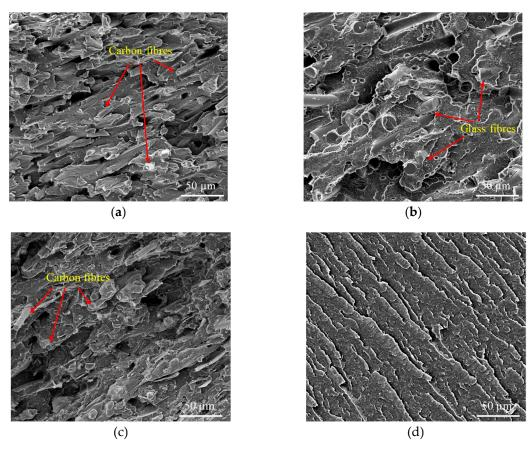
**Figure 1.** SEM images of fracture cross-section for polyetheretherketone (PEEK) and PEEK composites, (a) 30 wt % carbon fibre reinforced PEEK, (b) 30 wt % glass fibre reinforced PEEK, (c) each 10 wt % of PTFE, graphite and carbon fibre modified PEEK, (d) neat PEEK.
