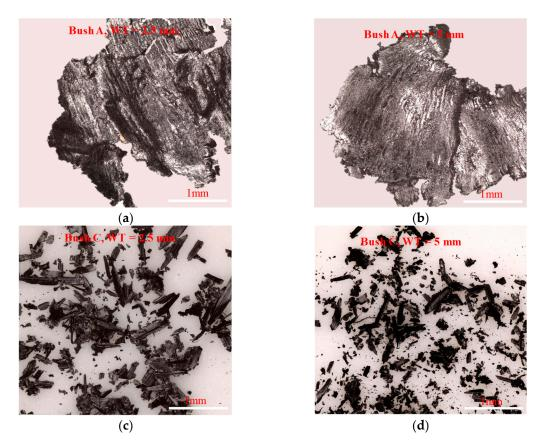
**Figure 6.** Typical debris observed from the wear test for (**a**) and (**b**) Bush A; (**c**) and (**d**) Bush C for wall thickness 2.5 and 5 mm, respectively. No wear debris observed from Bush B (glass fibre reinforced PEEK) and Bush D (unfilled PEEK).
