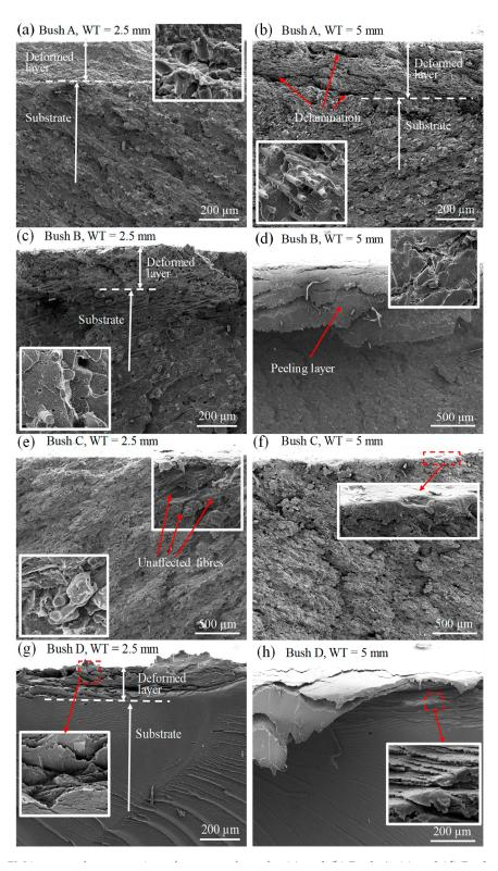
**Figure 8.** SEM images of cross section of worn surfaces for (**a**) and (**b**) Bush A, (**c**) and (**d**) Bush B, (**e**) and (**f**) Bush C, and (**g**) and (**h**) Bush D for wall thickness of 2.5 and 5 mm, respectively.
