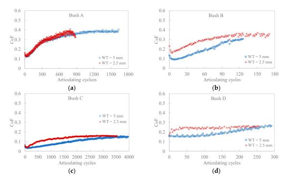
**Figure 4.** Typical evolution of CoF and recorded temperature varying with articulating cycles for (**a**) Bush A; (**b**) Bush B; (**c**) Bush C; (**d**) Bush D.
