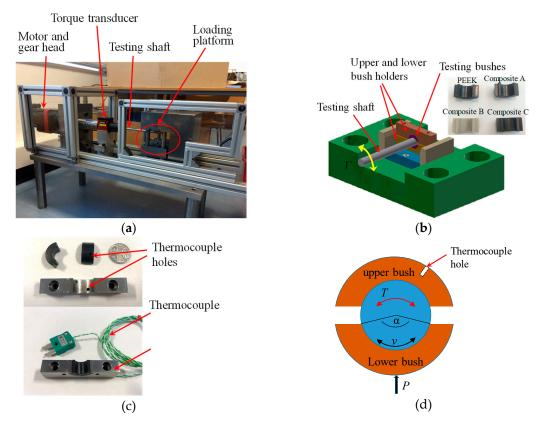
**Figure 2.** Pin joint test rig and bush specimen arrangement, (**a**) photo of the pin joint test rig; (**b**) loading platform with pin/bush assembly, bush halves located in two separate holders above and below the shaft, inset: bush specimens made of PEEK and PEEK composites; (**c**) thermocouple location; (**d**) contact geometry between shaft and bush halves subjected to normal load P applied from the lower bush, shaft oscillating speed v and required frictional torque T.
