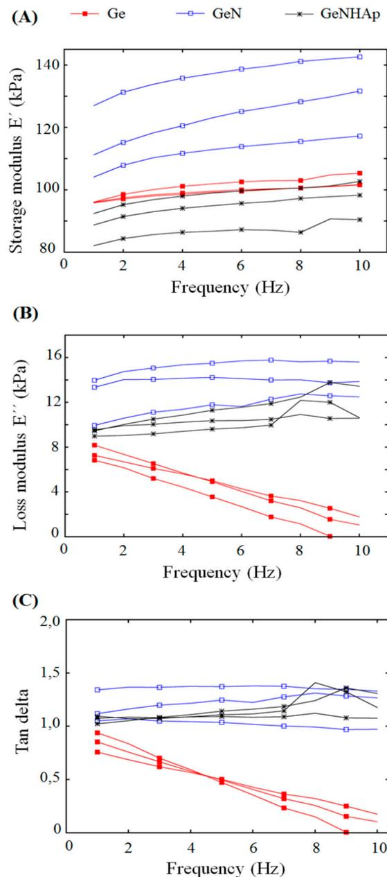
**Figure 9.** Viscoelastic properties of the 3D hybrid scaffolds (GeN, GeNHAp) and Ge freeze-dried samples determined with DMA. (A) Storage modulus as a function of frequency; (B) loss modulus as a function of frequency; (C) tangent of phase lag as a function of frequency.
