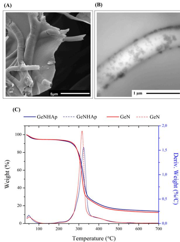
**Figure 3.** Analysis of fibers covered with HAp (GeNHAp). (A) SEM image presenting PLGA fibers embedded in the walls of freeze-dried Ge; (B) TEM image of a single fiber covered with HAp and embedded in freeze-dried gelatin solution; (C) thermogravimetric curves of the GeN and GeNHAp samples. The data show the differences in the thermal behavior of each type of sample and determine the HAp amount in the GeNHAp sample.
