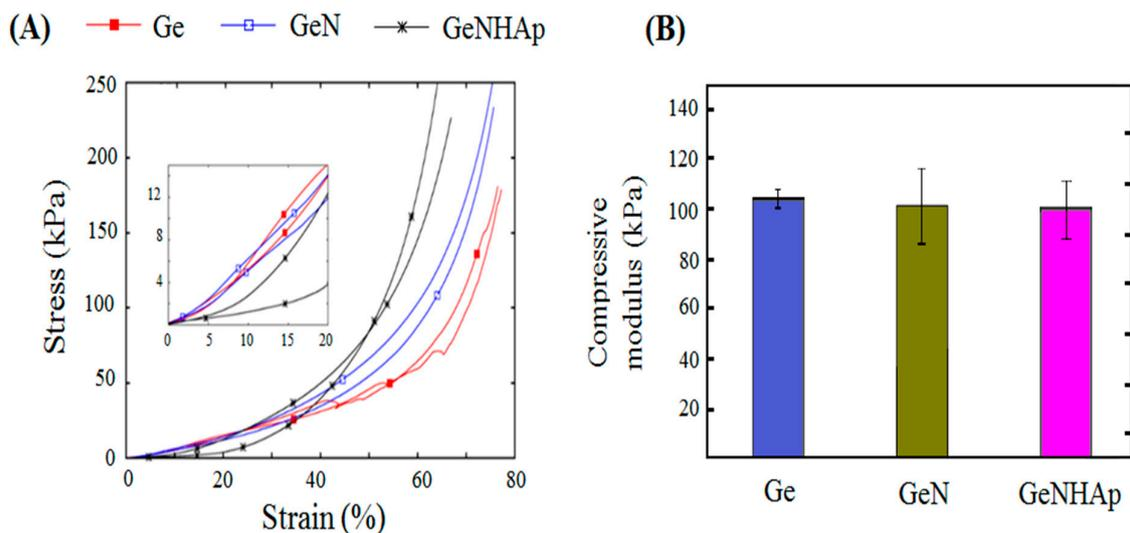
**Figure 8.** Stress–strain relationship of the 3D hybrid scaffolds (GeN, GeNHAp) determined with DMA: (A) compression stress–strain response of the analyzed 3D scaffolds; (B) compressive moduli of analyzed scaffolds.
