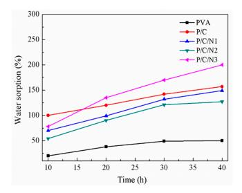
**Figure 6.** Water sorption of PVA, P/C, P/C/N1, P/C/N2, and P/C/N3 composite films.
