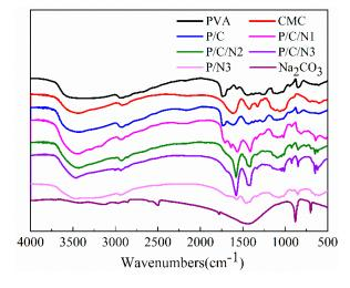
Figure 1. Fourier-transform infrared (FTIR) spectra of Na<sub>2</sub>CO<sub>3</sub> and the obtained composite films.
