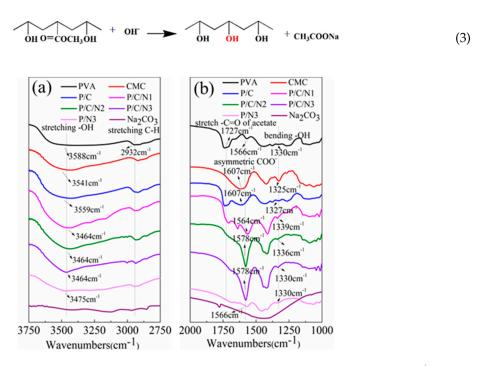
**Figure 2.** FTIR spectra of  $Na_2CO_3$  and the obtained composite films: (a) region from 3750 cm<sup>-1</sup> to 2750 cm<sup>-1</sup>; (b) region from 2000 cm<sup>-1</sup> to 1000 cm<sup>-1</sup>.
