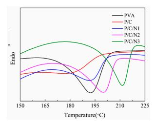
Figure 4. Differential scanning calorimetry (DSC) curves of the obtained composite films.
