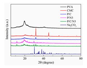
Figure 3. X-ray diffraction (XRD) patterns of Na<sub>2</sub>CO<sub>3</sub> and the obtained composite films.
