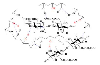
Figure 9. The reaction mechanism for PVA, CMC, and Na<sub>2</sub>CO<sub>3</sub>.
