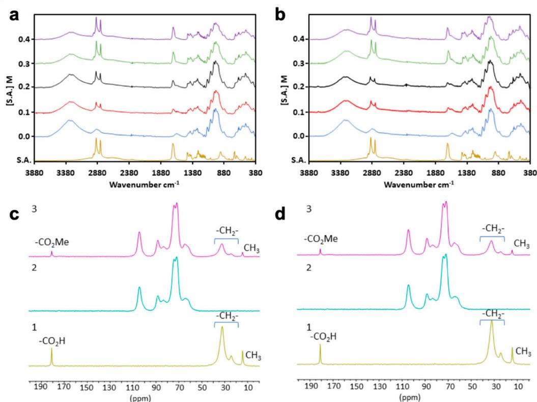
**Figure 11.** FTIR and NMR spectra for flax modified by stearic acid. (a) (Ethanol) and (b) (toluene) FTIR spectra ([SA] = 0.1, 0.2, 0.3, and 0.4 M). <sup>13</sup>C CP/MAS NMR spectrum of stearic acid 1 (SA), flax fabric (blue) 2, and, in purple, the flax fabric treated with 0.4 M of SA in ethanol (c) and in toluene (d).
