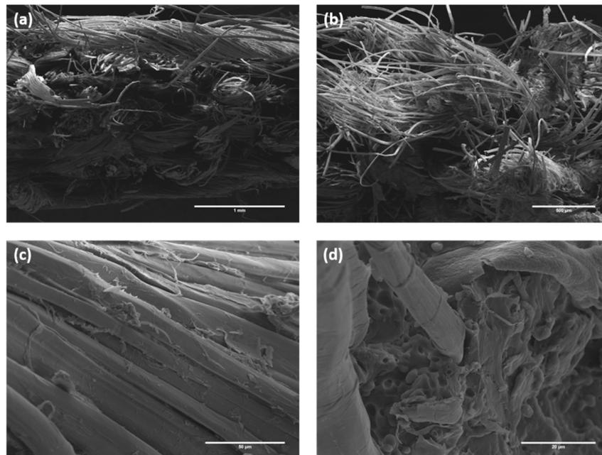
**Figure 5.** SEM micrographs of the fracture surfaces of PP/Flax composites at different magnifications.
