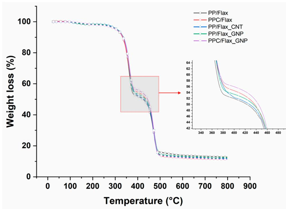
Figure 10. Thermograms for the different PP/flax composites.
