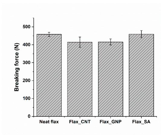
**Figure 4.** Breaking forces of untreated and surface-modified flax fabrics.
