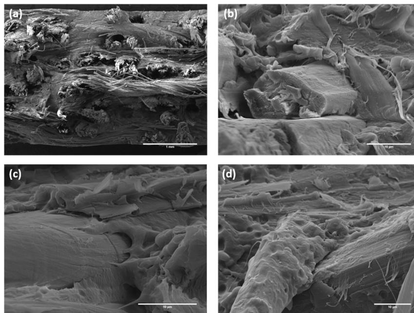
**Figure 6.** SEM micrographs of the fracture surface of PPC (PP modified with coupling agent)/Flax composites at different magnifications.
