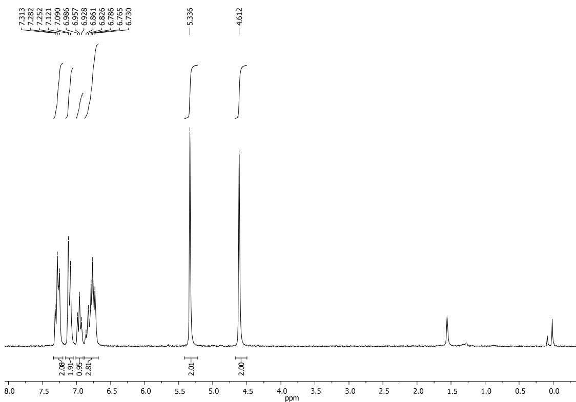
**Figure S31.**  $^1\text{H}$  NMR (250 MHz) spectrum of **6** in  $\text{CDCl}_3$ .
