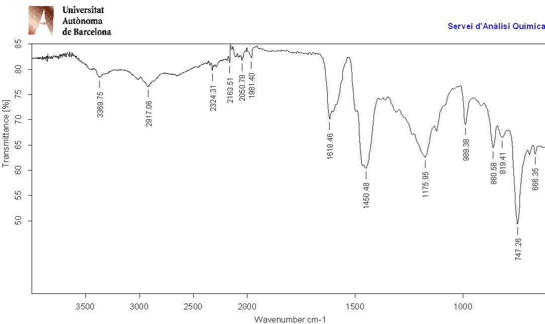
**Figure S54.** IR (ATR)  $\nu$  (cm<sup>-1</sup>) of polymer derived from 6.
