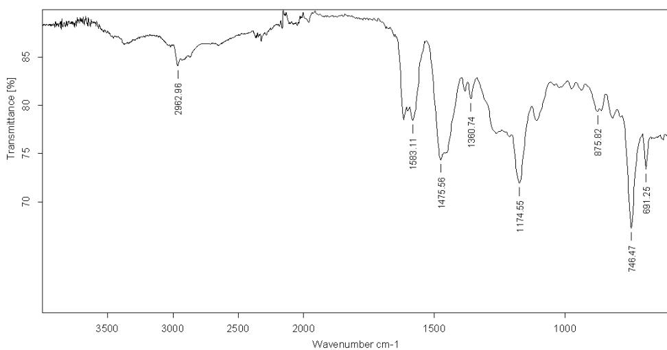
**Figure S57.** IR (ATR)  $\nu$  ( $\text{cm}^{-1}$ ) of polymer derived from **BPA-a**.
