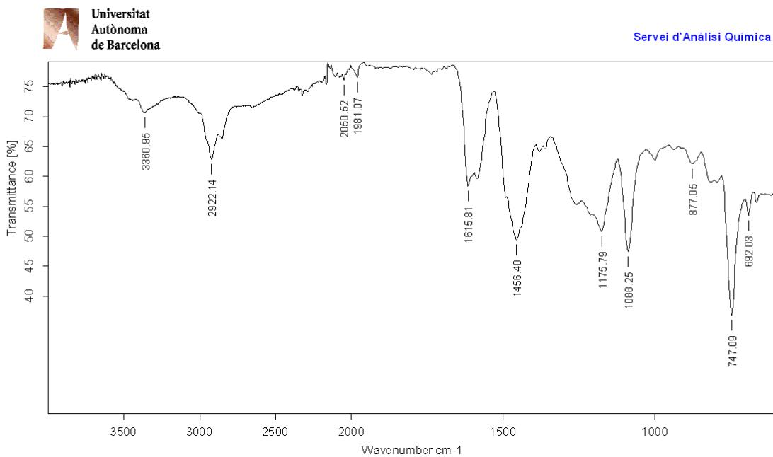
**Figure S52.** IR (ATR)  $\nu$  ( $\text{cm}^{-1}$ ) of polymer derived from **4**.
