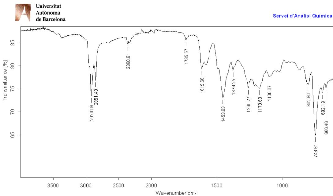
**Figure S50.** IR (ATR)  $\nu$  ( $\text{cm}^{-1}$ ) of polymer derived from 2.
