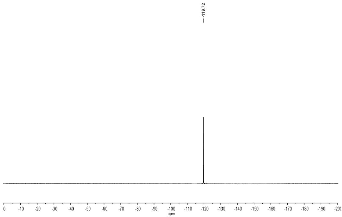
**Figure S44.**  $^{19}\text{F}$  NMR (235.2 MHz) spectrum of **8** in  $\text{CDCl}_3$ .
