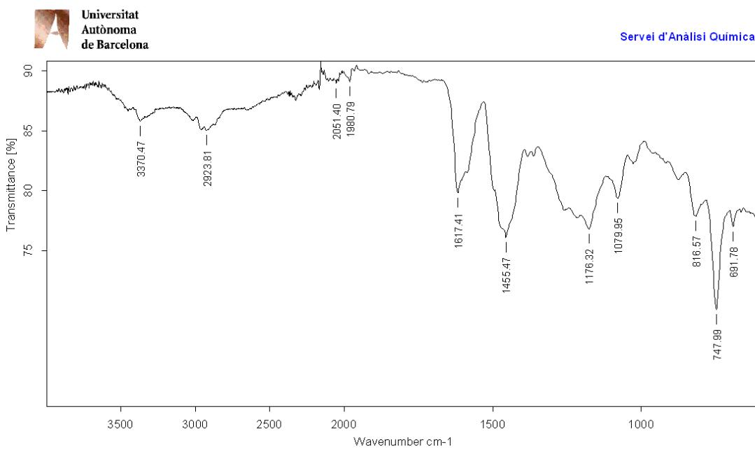
**Figure S56.** IR (ATR)  $\nu$  ( $\text{cm}^{-1}$ ) of polymer derived from 8.
