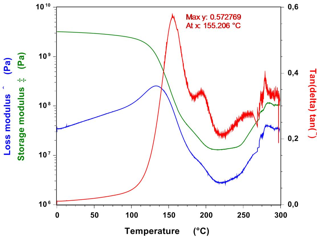
Figure S15. DMA thermogram of **2a** and **2b**.
