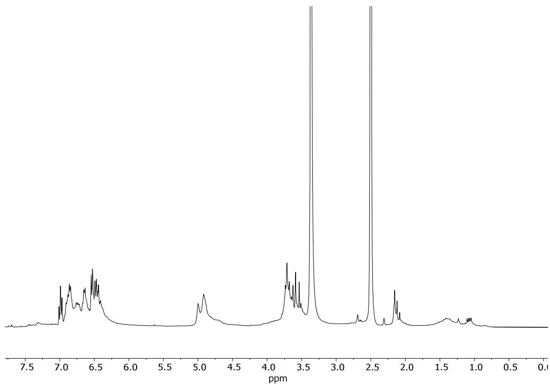
**Figure S60.** <sup>1</sup>H NMR (360 MHz) of **polymer** derived from **3** in DMSO-d<sub>6</sub>.
