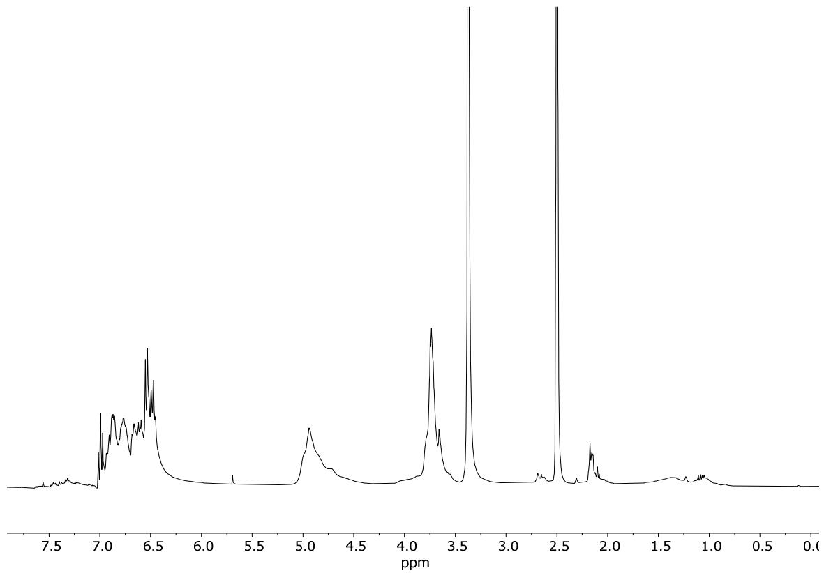
**Figure S63.** <sup>1</sup>H NMR (360 MHz) of polymer derived from **6** in DMSO-d<sub>6</sub>.
