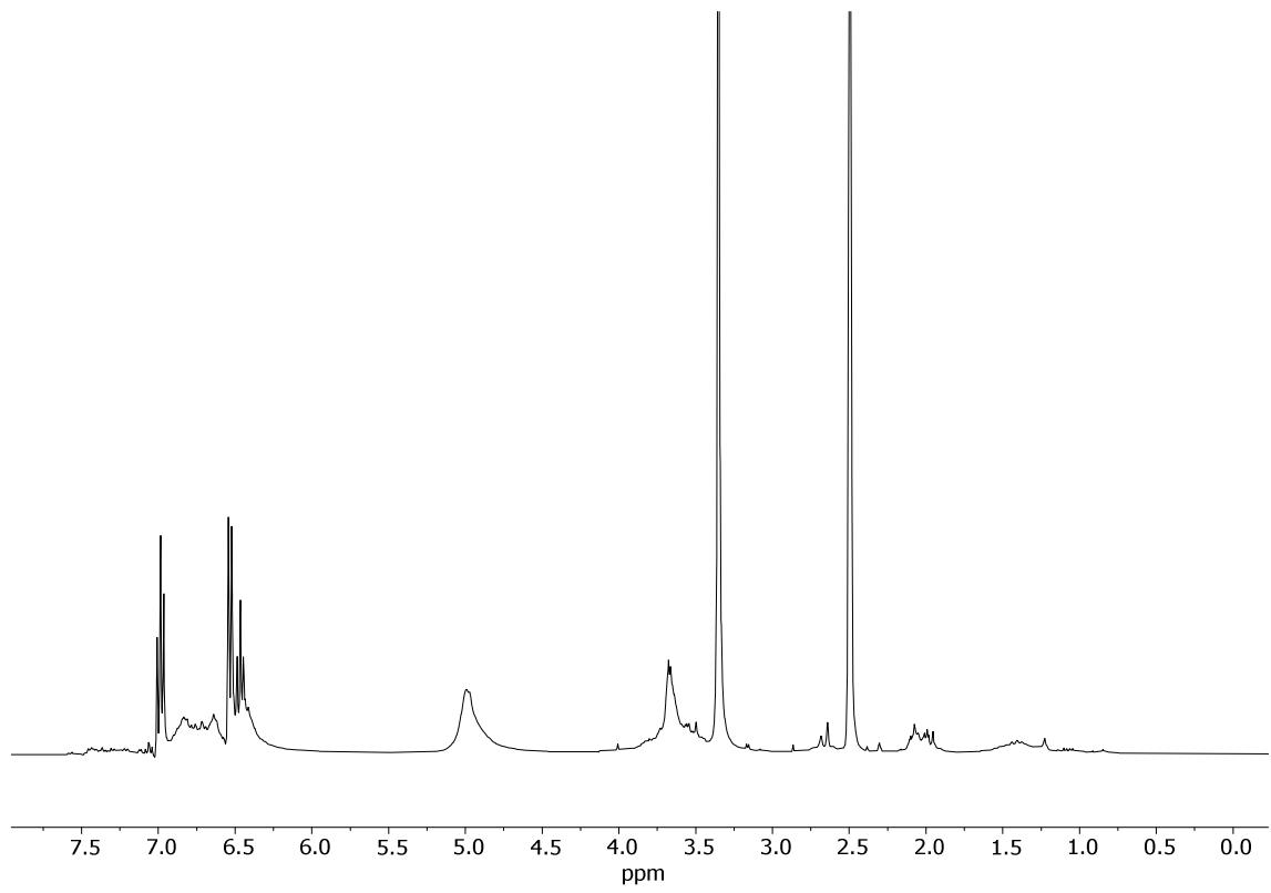
**Figure S62.** <sup>1</sup>H NMR (360 MHz) of polymer derived from **5** in DMSO-d<sub>6</sub>.
