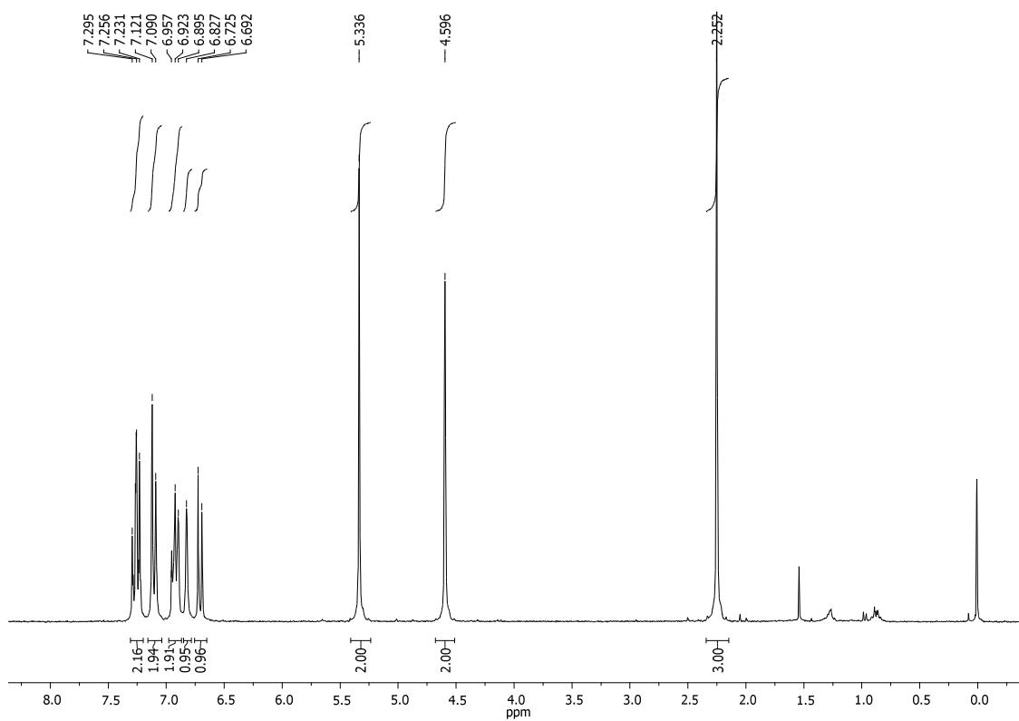
**Figure S1.** <sup>1</sup>H NMR (250 MHz) spectrum of **1** in CDCl<sub>3</sub>.
