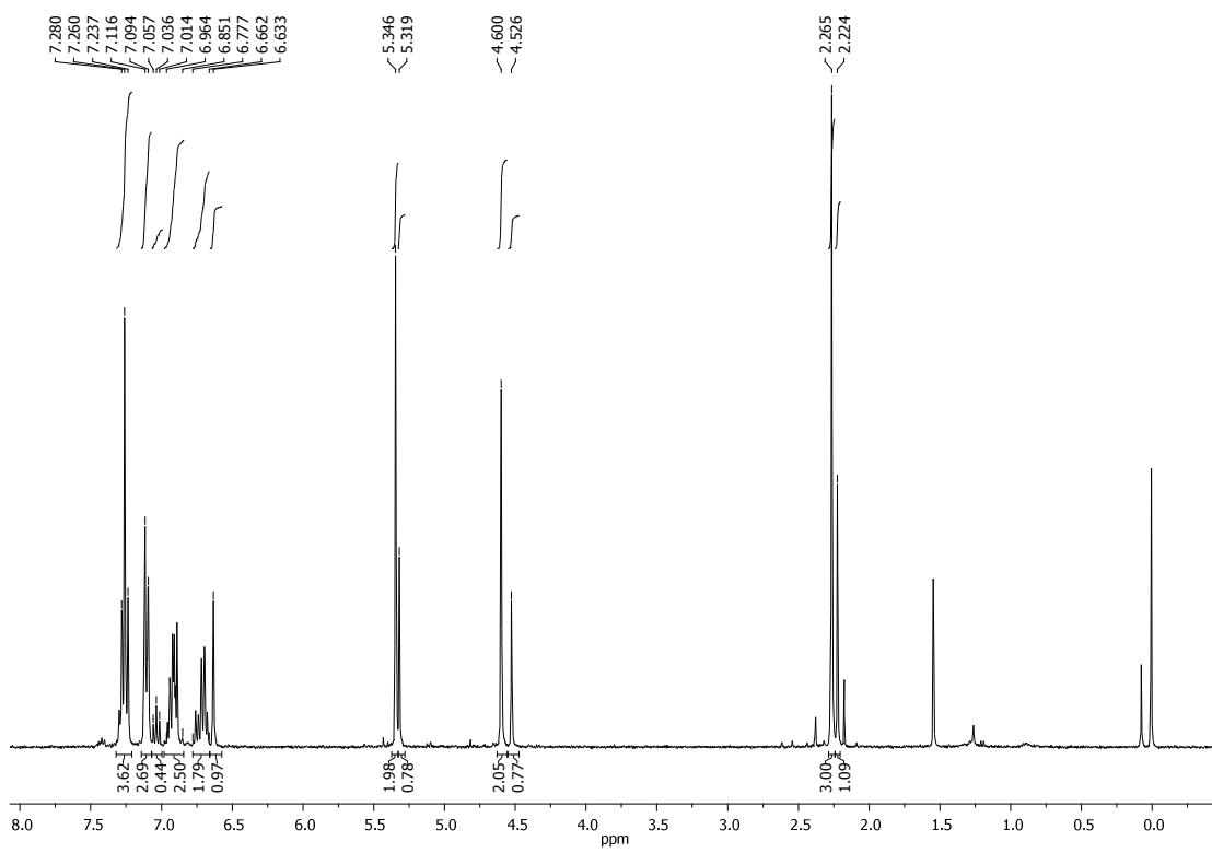
**Figure S6.**  $^1\text{H}$  NMR (360 MHz) spectrum of **2a** and **2b** in  $\text{CDCl}_3$ .
