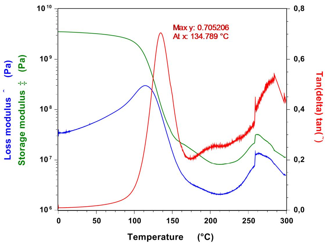
Figure S20. DMA thermogram of 3.
