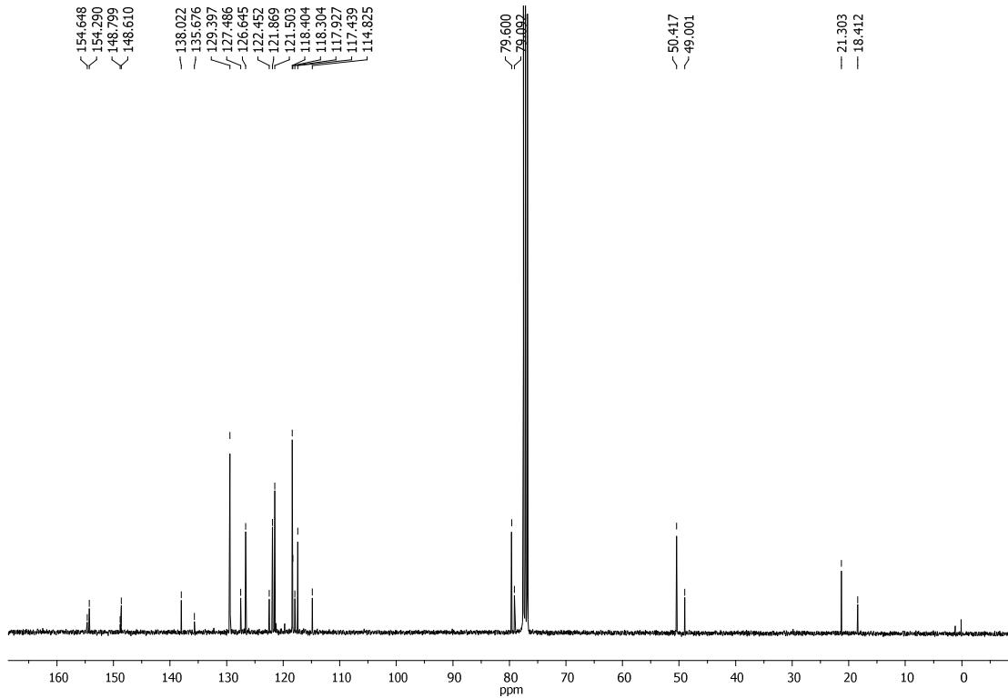
**Figure S7.**  $^{13}\text{C}$  NMR (90.5 MHz) spectrum of **2a** and **2b** in  $\text{CDCl}_3$ .
