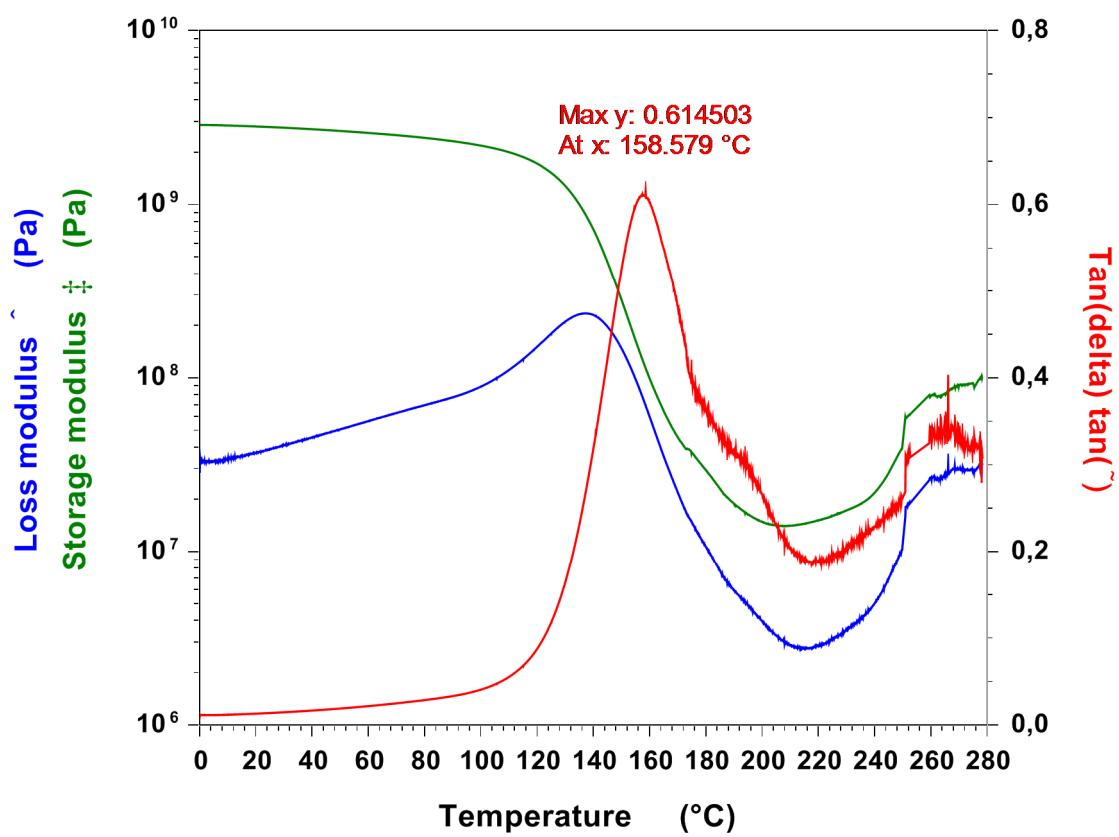
Figure S25. DMA thermogram of 4.
