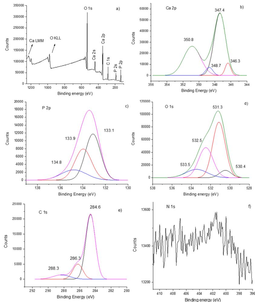
**Figure 3.** XPS data of HAPCs coatings deposited on Si substrates at  $5 \times 10^{-3}$  mbarr Ar gas working pressure: (a) survey spectrum; (b) Ca 2p; (c) P 2p; (d) O 1s; (e) C1s; and (f) N 1s high-resolution lines.
