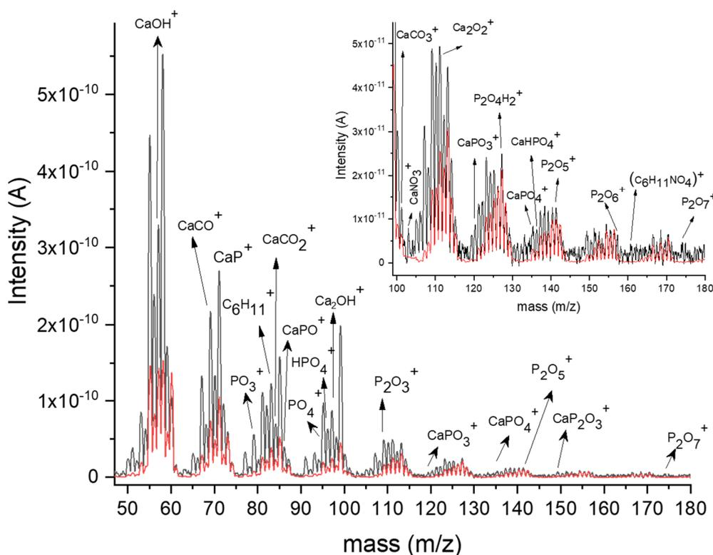
**Figure 2.** Mass spectrum of the residual gas extracted from the vacuum chamber during plasma on (black line) and plasma off (red line).
