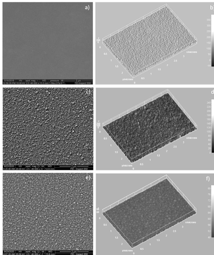
**Figure 6.** SEM images of HApCs coatings at: (a)  $p = 2 \times 10^{-3}$  mbarr; (c)  $p = 5 \times 10^{-3}$  mbarr; (e)  $p = 1.2 \times 10^{-2}$  mbarr; 3D images of: (b) Figure 6a; (d) Figure 6c; (f) Figure 6e; performed with ImageJ software.
