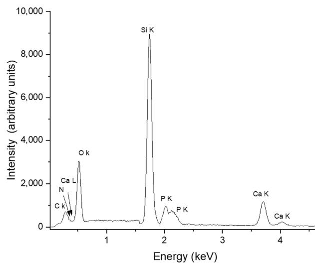
**Figure 7.** EDS spectrum of HApCs layers generated at  $5 \times 10^{-3}$  mbarr Ar gas working pressure.
