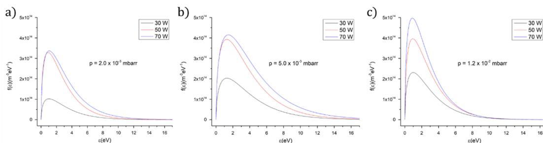
Figure 1. Dependence of electron energy distribution function on applied radio frequency (rf) power for: (a)  $p = 2 \times 10^{-3}$  mbarr; (b)  $p = 5 \times 10^{-3}$  mbarr; (c)  $p = 1.2 \times 10^{-2}$  mbarr.
