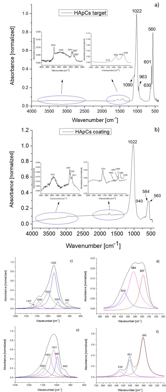
**Figure 4.** FTIR spectra of: (a) HApCs target; (b) HApCs coating deposited on Si substrate at  $5 \times 10^{-3}$  mbar Ar gas working pressure; FTIR deconvoluted spectra of HApCs target and of HApCs coating deposited on Si substrate at  $5 \times 10^{-3}$  mbar Ar gas working pressure in: (c,e) 1200–850  $\text{cm}^{-1}$  range; (d,f) 680–500  $\text{cm}^{-1}$  range.
