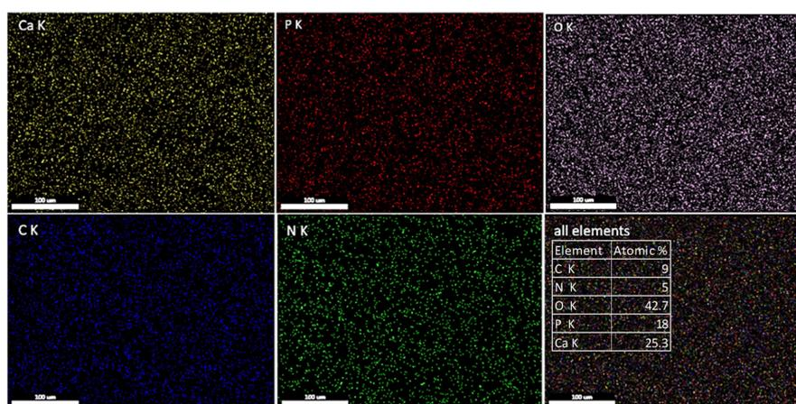
Figure 8. 2D SEM-EDS elemental mapping of the HApCs coating.
