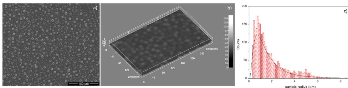
**Figure 5.** (a) Survey SEM image of HApCs coatings generated at  $5 \times 10^{-3}$  mbarr Ar gas working pressure; (b) 3D image of Figure 1 performed with ImageJ software; (c) histogram of particle sizes.
