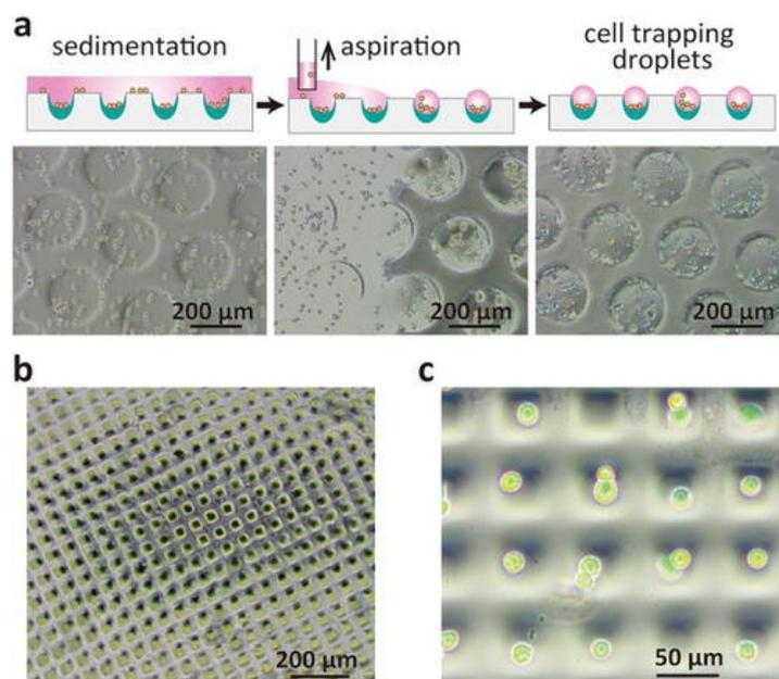
**Figure 8.** Schematic illustration of the cell trapping mechanism in polydimethylsiloxane (PDMS) microwells and the corresponding micrographs in (a) 200  $\mu\text{m}$  and (b) 35  $\mu\text{m}$  square microwell arrays. (c) Single-cell trapping demonstrated using a combination of bright field microscopy and fluorescence imaging. (Reprinted with permission from [68] Copyright (2018), American Institute of Physics).
