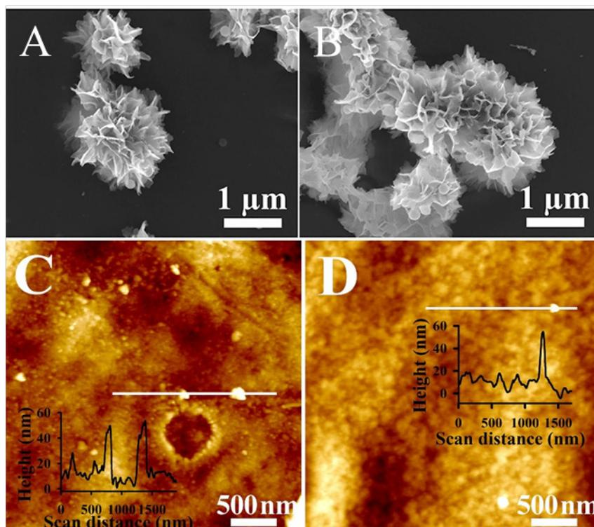
**Figure 5.** Scanning electron microscopy (A,B) and atomic force microscopy (C,D) images of poly(styryl bisphosphonate) (poly(StBP))-6, and poly(StBP)-40 (D) films, respectively, where “6” and “40” represent the thickness of the Mayer rod (6 and 40  $\mu\text{m}$ ) used to spread the polymer solution. (Reprinted with permission from [62] Copyright (2020), Elsevier).
