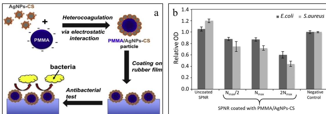
**Figure 4.** (a) Schematic illustration of polymethyl methacrylate/chitosan-silver (PMMA/AgNPs-CS) coating and its antibacterial activity; (b) optical density of suspension of *Escherichia coli* and *Staphylococcus aureus*. (Reprinted with permission from [56] Copyright (2019), Elsevier).
