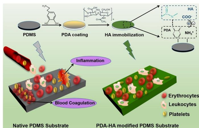
**Figure 7.** Schematic illustration of polydimethylsiloxane (PDMS) surface modification using hyaluronic acid and polydopamine (HA/PDA) composite coatings. (Reprinted with permission from [67]. Copyright (2017), American Chemical Society).
