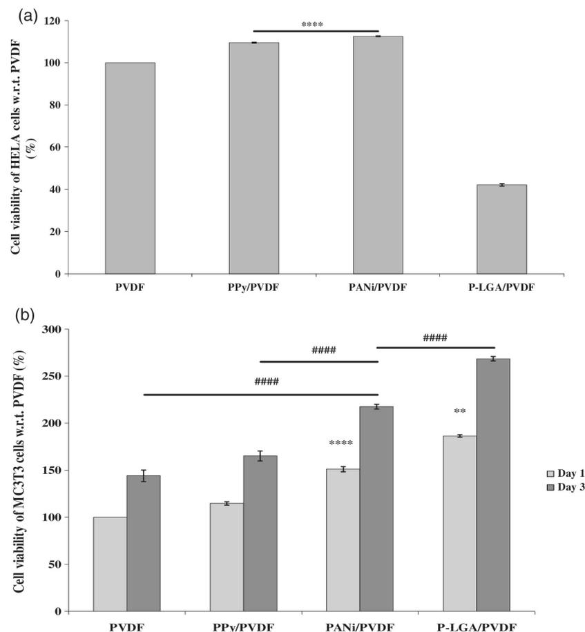
**Figure 2.** Viability of (a) HeLa cells and (b) MC3T3 cells on PVDF and PVDF:CP electrospun fibers (control: PVDF). \*\* and \*\*\*\* signifies  $p < 0.01$  (1d) and  $p < 0.0001$  (1d), respectively, for both HeLa and MC3T3 culture (1d); ##### signifies  $p < 0.0001$  (3d). CP, conducting polymers; PVDF, poly(vinylidene fluoride) (Reprinted with permission from [47] Copyright (2020), John Wiley and Sons).
