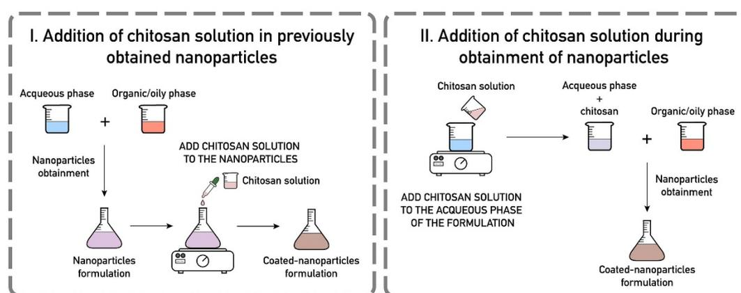
**Figure 9.** Different approaches of chitosan coatings for nanoparticles. (Reprinted with permission from [90] Copyright (2020), Elsevier).
