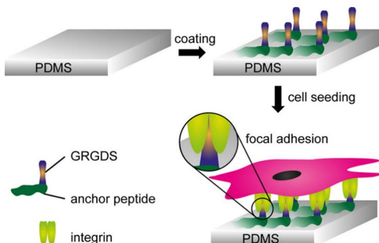
**Figure 6.** Schematic illustration of polydimethylsiloxane (PDMS) coating using engineered anchor peptides fused to the cell-adhesive peptide sequence (glycine-arginine-glycine-aspartateserine, GRGDS). (Reprinted with permission from [63] Copyright (2019), American Chemical Society).
