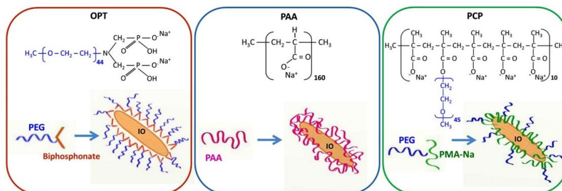
**Figure 10.** Schematic illustration of iron oxide nanorods coated with linear bisphosphonate–poly(ethylene glycol) (OPT), polyacrylic sodium salt (PAA), and polymethacrylate backbone/PEG side chain comb polymer (PCP). (Reprinted with permission from [97]. Copyright (2018), American Chemical Society).
