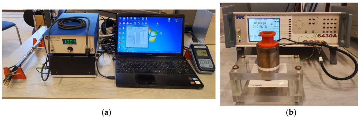
**Figure 5.** Measurement of dielectric properties: (a) voltage response measurement on a PVC cable sample; (b) measurement of PVC films by cylindrical copper electrodes by Wayne-Kerr 6430A impedance analyzer.
