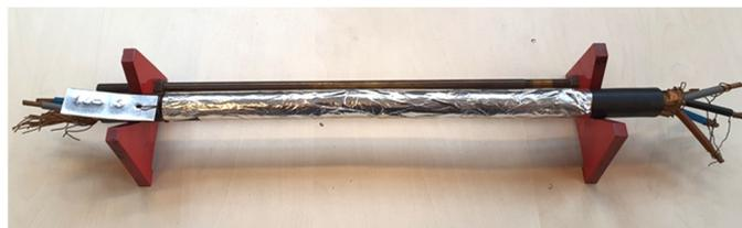
**Figure 2.** Cable sample prepared for measurement. The inner conductor is the screen tape connected to all core conductors; the outer one is an aluminum foil wrapped around the cable.
