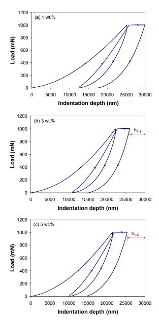
**Figure 5.** Experimental load-depth curves for 2-cycle indentation on the PP/MWCNT nanocomposites at 2000 mN/min loading/unloading rate and 300 s holding time.
