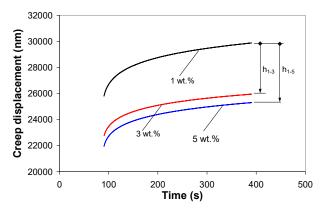
**Figure 7.** Indentation creep displacement curves for the PP/MWCNT nanocomposites (holding stage of the 2-cycle indentation test).
