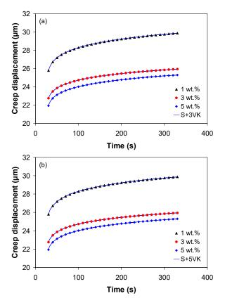
**Figure 9.** Comparison between experimental creep displacement and prediction based on the S + nVK model with (**a**) three VK units and (**b**) five VK units (predictions are shown as solid lines).
