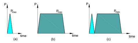
**Figure 1.** Schematic representation of the indentation loading profile for (a) 2-step, (b) 3-step, and (c) 2-cycle indentation tests.
