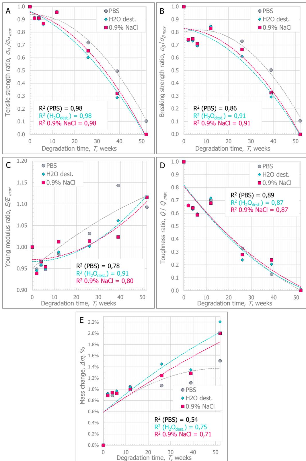
**Figure 2.** Tendencies of the changes in material parameters during degradation: (A) Tensile strength ratio; (B) Breaking strength ratio; (C) Young modulus ratio; (D) Toughness ratio; (E) Mass change.
