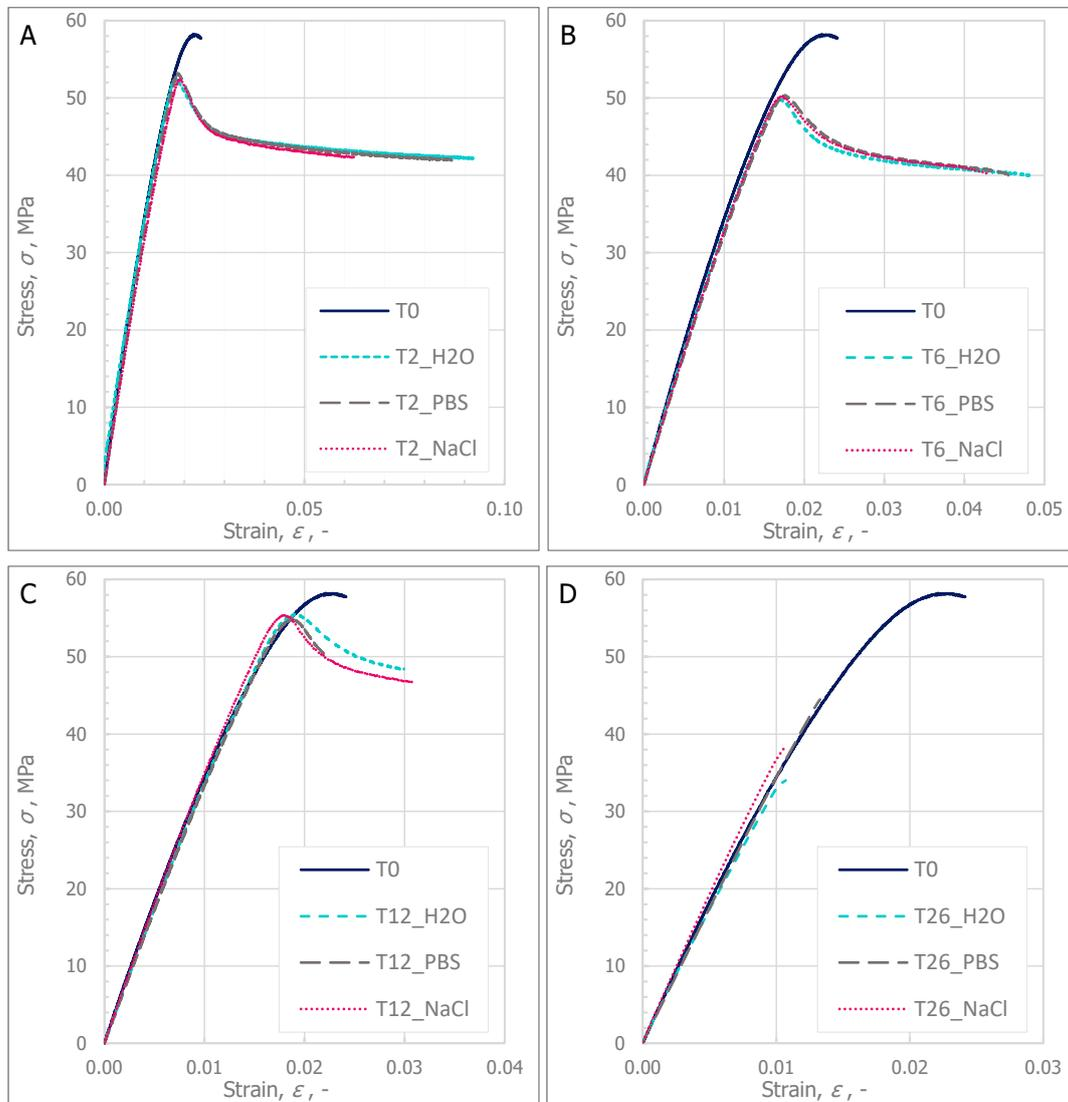
**Figure 1.** The stress–strain curves of the specimens during degradation in various mediums: (A) Comparison between specimens before degradation (T0) and after two weeks of degradation; (B) Comparison between specimens before degradation and after six weeks of degradation; (C) Comparison between specimens before degradation and after twelve weeks of degradation; (D) Comparison between specimens before degradation and after twenty-six weeks of degradation.
