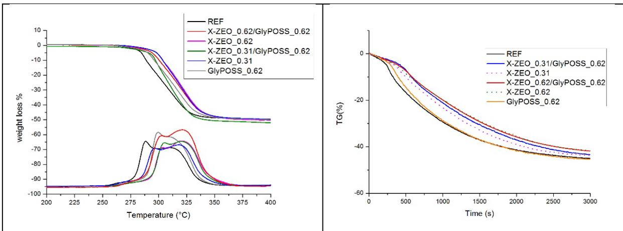
Figure S1: TGA analyses of reference P-PVC and X-type zeolite and X-type zeolite/GlyPOSS formulations in the compositional range 0.31–0.62 phr, in ramp heating 10°C/min, Ar flow (20 mL/min) from RT to 800°C (left) and isothermal measurements (Ar, 265°C) (right).
