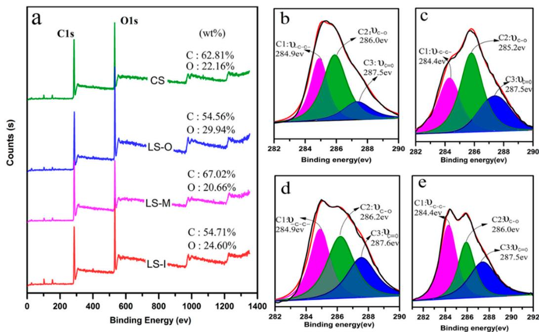
**Figure 8.** (a) X-ray photoelectron spectroscopy (XPS) survey spectra of four samples and C1s spectra of (b) CS, (c) LS-O, (d) LS-M, and (e) LS-I.
