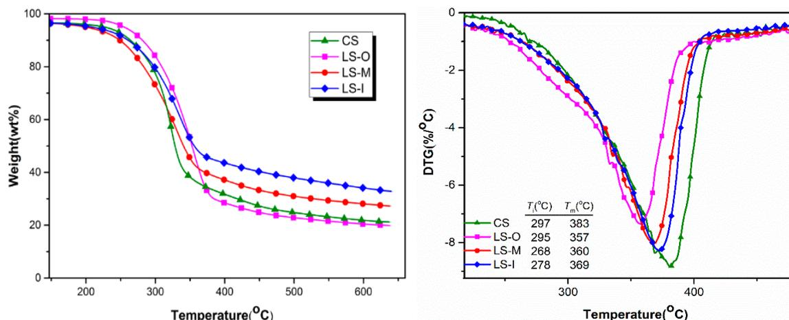
**Figure 5.** Thermal Gravity Analysis (TG)/Differential thermal gravity (DTG) analysis curves of different samples. Notes:  $T_i$  and  $T_m$  refer to the temperature where starting decomposition and the maximum mass loss occur.
