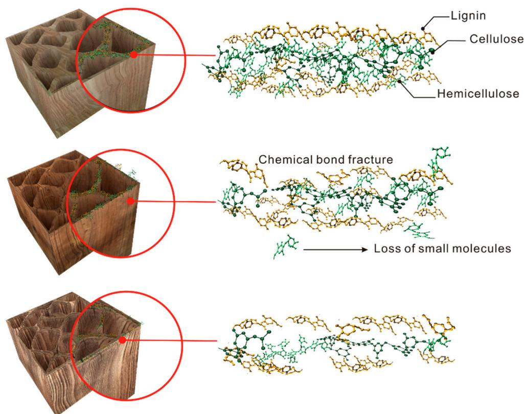
**Figure 7.** Schematic illustration of the change of three major components in the timber in the ancient buildings in the natural aging process.
