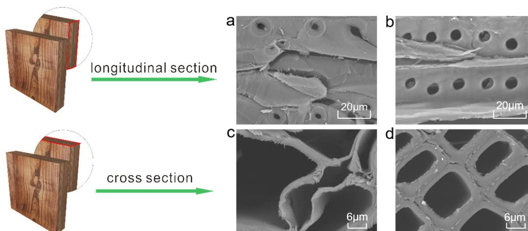
**Figure 6.** SEM images of the cross-section topography of (a) and (c) the outer layer of ancient timbers, (b) and (d) the control fresh samples.
