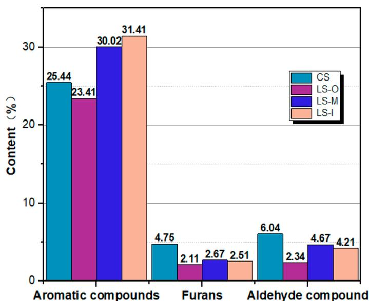
**Figure 4.** Main pyrolysis products contents for CS LS-O LS-M and LS-I obtained from Py-GC/MS measurements.
