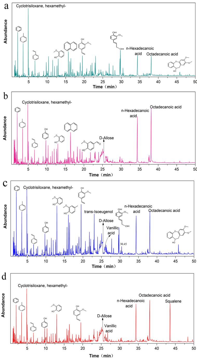
Figure 3. Detailed Py-GC/MS data for (a) CS, (b) LS-O, (c) LS-M, and (d) LS-I.
