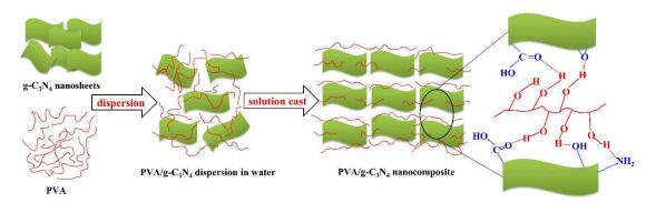
**Figure 2.** Schematic illustration of nanocomposite preparation and the interaction between  $g-C_3N_4$  nanosheets and poly(vinyl alcohol (PVA).
