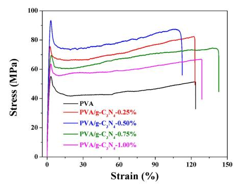
Figure 7. Stress-strain curves of pure PVA and PVA/g-C<sub>3</sub>N<sub>4</sub> nanocomposites.
