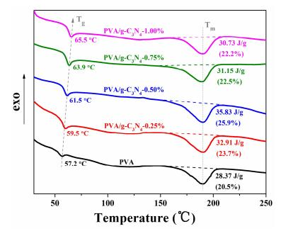
Figure 6. DSC curves of pure PVA and PVA/g-C<sub>3</sub>N<sub>4</sub> nanocomposites.
