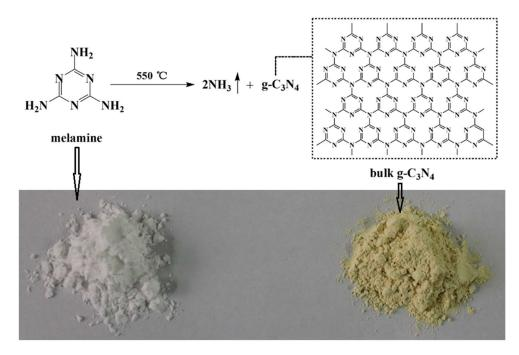
Figure 1. Thermal condensation process from melamine to bulk g-C<sub>3</sub>N<sub>4</sub>.
