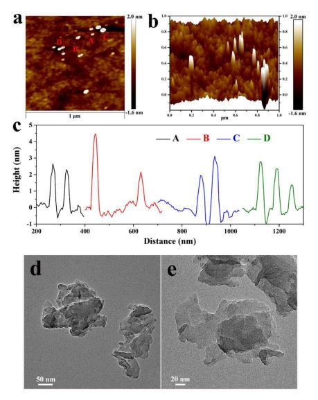
**Figure 3.** Atomic force microscope (AFM) (**a**) top view, (**b**) height topography image, (**c**) height trace curves of g-C<sub>3</sub>N<sub>4</sub> nanosheets placed on a silicon substrate, and (**d**,**e**) TEM images of g-C<sub>3</sub>N<sub>4</sub> nanosheets.
