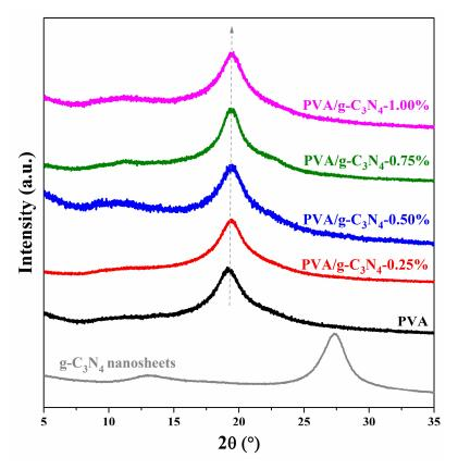
Figure 5. XRD curves of  $PVA/g-C_3N_4$  nanocomposites with various  $g-C_3N_4$  contents.
