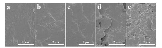
**Figure 4.** SEM images of tensile fractured surface for (**a**) pure PVA and PVA/g-C<sub>3</sub>N<sub>4</sub> nanocomposites with g-C<sub>3</sub>N<sub>4</sub> content of (**b**) 0.25 wt %, (**c**) 0.50 wt %, (**d**) 0.75 wt % and (**e**) 1.00 wt %.
