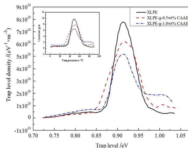
**Figure 3.** Thermally stimulated depolarization current (TSDC) spectrum (inset panel) and derived trap levels distribution of XLPE and XLPE-g-CAAE.
