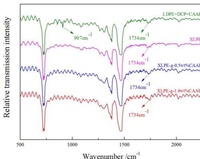
**Figure 1.** Fourier-transform infrared (FT-IR) of crosslinked polyethylene (XLPE), LDPE + Dicumyl Peroxide (DCP) + chloroacetic acid allyl ester (CAAE) and crosslinked polyethylene grafted with chloroacetic acid allyl ester (XLPE-g-CAAE).
