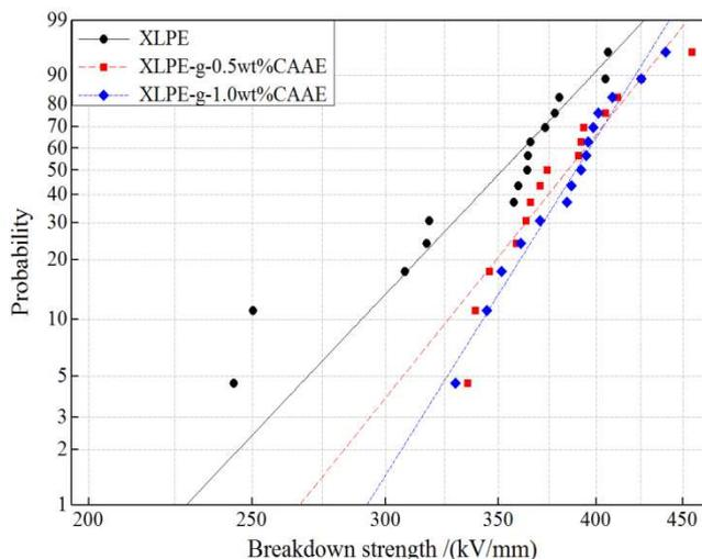
**Figure 6.** DBS statistics with fitted 2-parameter Weibull distribution for XLPE and XLPE-g-CAAE.
