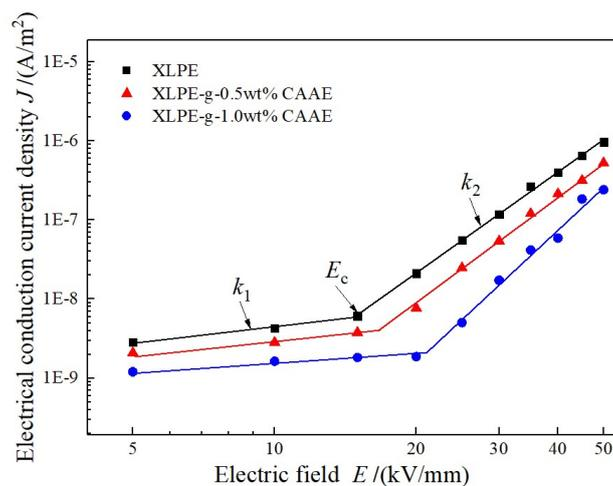
**Figure 5.** Electrical conduction current density of XLPE-g-CAAE varying with applied electric field.
