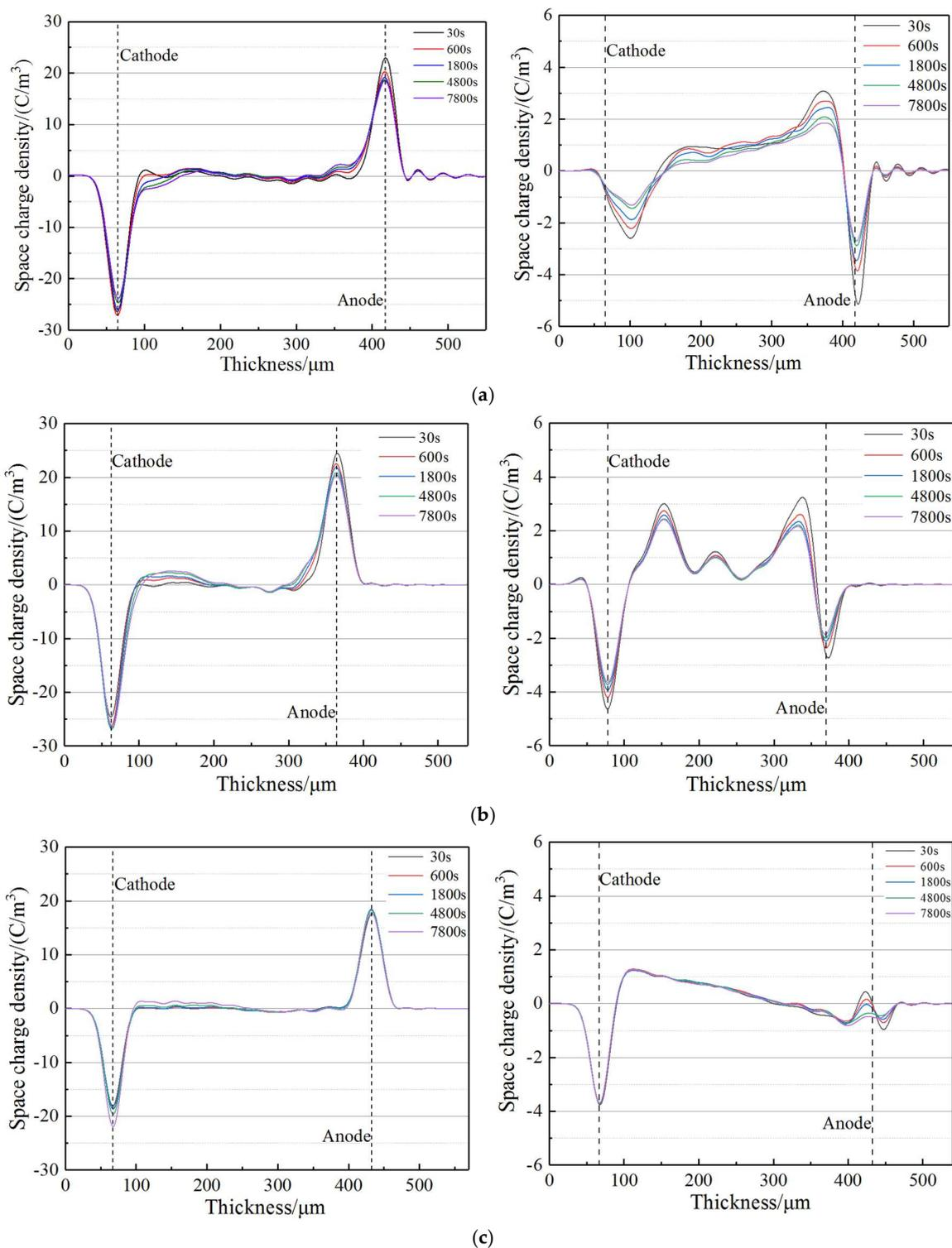
**Figure 2.** Space charge distribution in (a) XLPE, (b) XLPE-g-0.5wt%CAAE, and (c) XLPE-g-1.0wt%CAAE under applied DC electric field 40 kV/mm (left panels) and with electrode short connection (right panels).
