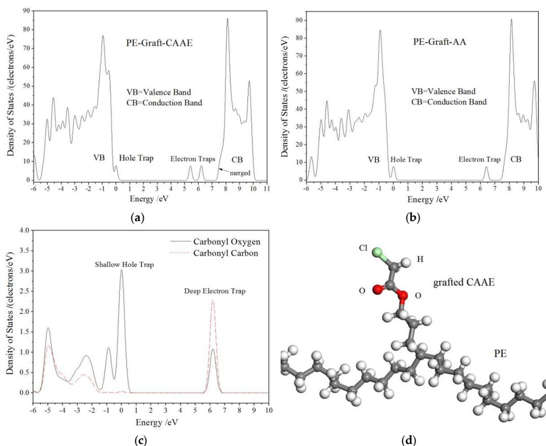
**Figure 4.** First-principles calculated (a) density of state (DOS) of CAAE grafted polyethylene (PE-g-CAAE), (b) DOS of allyl acetate-grafted-PE (PE-g-AA), (c) projected density of states (PDOS) on the oxygen and carbon of C=O in PE-g-AA, (d) schematic molecular structure in relaxation (after geometry optimization) of PE-g-CAAE. The highest occupied molecular orbital (HOMO) is referenced as energy zero and smearing is 0.1 eV.
