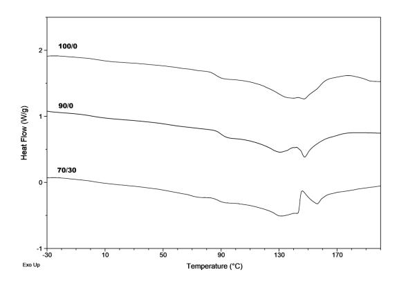
DSC plot of P(3HB-co-4HB)/cork composites (100/0), (90/10), (70/30) after 21 days of degradation in the respirometer.
