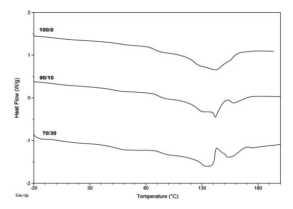
DSC plot of P(3HB-co-4HB)/cork composites (100/0), (90/10), (70/30) after 21 days of degradation in the container.
