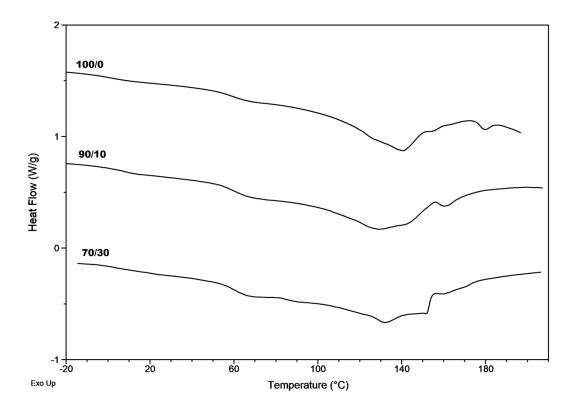
DSC plot of P(3HB-co-4HB)/cork composites (100/0), (90/10), (70/30) after 21 days of degradation in the water.
