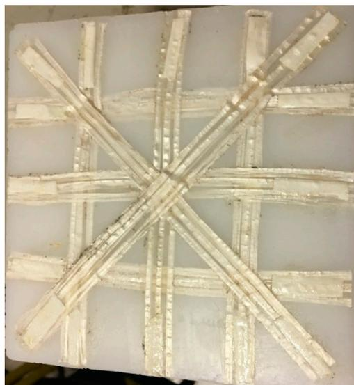
Figure 2. Picture of rotational molded homo-composite prototype.
