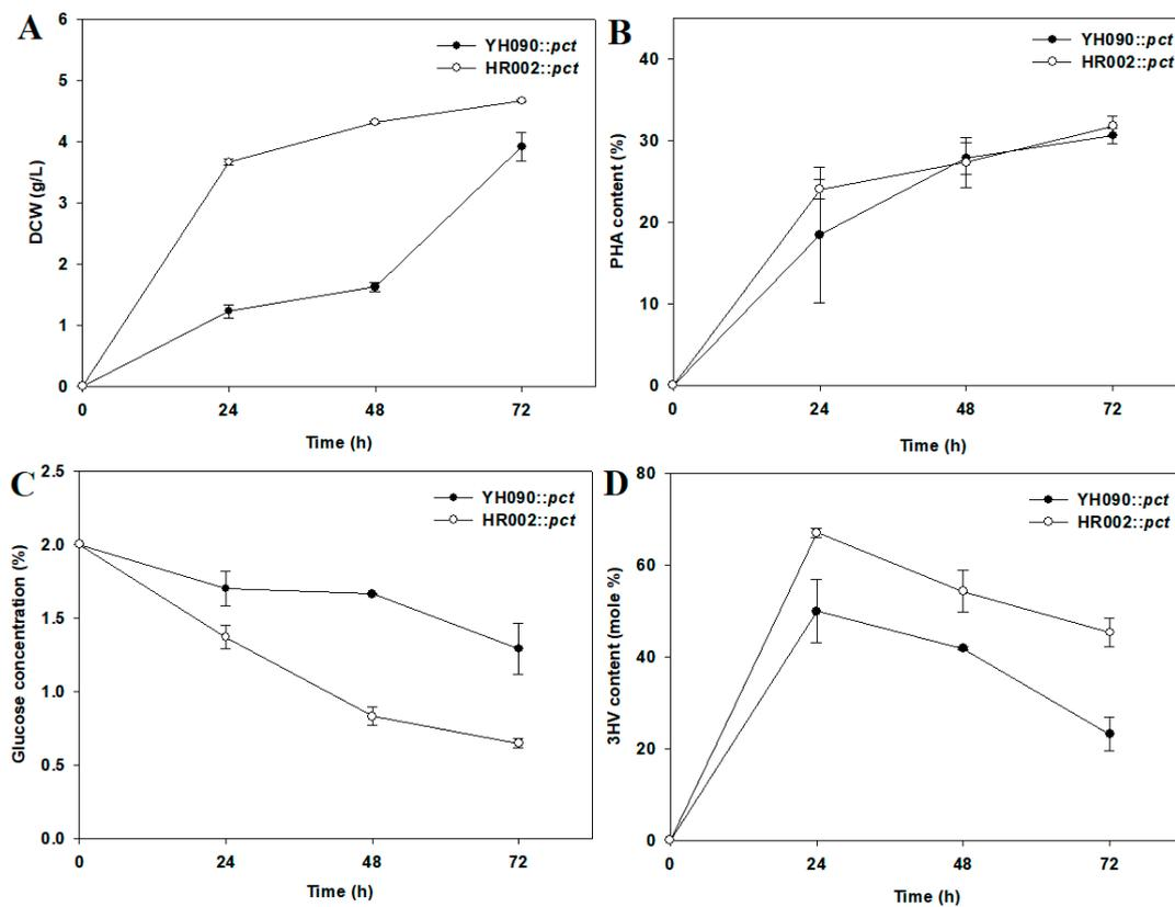
**Figure 5.** Monitoring of PHBV production in *YH090::pct* and *HR002::pct*: (A) DCW (dry cell weight, g/L); (B) PHA content (wt/wt %); (C) Glucose concentration (g/L); and (D) 3-hydroxyvalerate monomer content (mol %). Cell cultivation was conducted for 72 h in M9 minimal medium containing 2% glucose and 0.15% sodium propionate. Error bars represent the standard deviations of two replicates.
