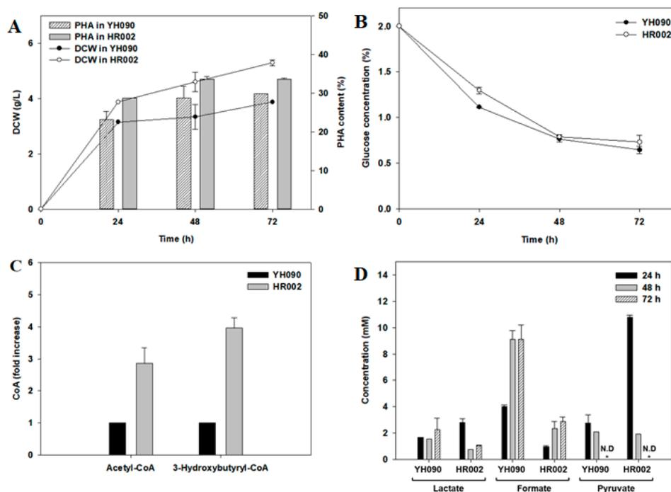
**Figure 3.** Polyhydroxybutyrate (PHB) production in engineered *E. coli* over time: (A) DCW (dry cell weight, g/L) and PHB content (wt/wt %); (B) glucose concentration (g/L); (C) relative amount of CoA metabolites (fold increase); and (D) secreted organic acid concentration [40]. Cell cultivation was conducted for 72 h in M9 minimal medium containing 2% glucose as a sole carbon source. CoA metabolites were measured at 6 h. Error bars represent the standard deviations of two replicates.
