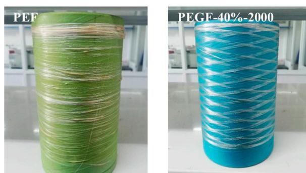
**Figure 20.** PEF and PEGF-40%-2000 monofilament.
