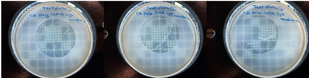
The photos of M1, M1b and M1c showed that after 24 h of incubation, the pure CA and the transitional membranes showed slight suppression of growth, but bacteria were still able to grow on the agar. The slight suppression is likely due to the shift in metabolism caused by the presence of membranes reducing the direct contact of agar with air, decreasing the availability of oxygen to serve as a terminal electron acceptor, therefore slowing the growth of bacteria and production of pigment.
