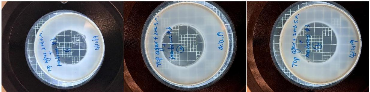
Photos of M2 and M3 showed an unambiguous inhibition of bacterial growth. M2 was observed to be more effective than M1, M1b and M1c, while M3 showed the best antimicrobial performance of all the membranes. The M3 plates showed a clearing spot visually indistinguishable from the negative control, thus, M3 completely suppressed the growth of *Serratia marcescens*.
