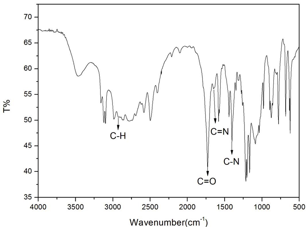
Figure S2. FT-IR spectrum of EC-g3
