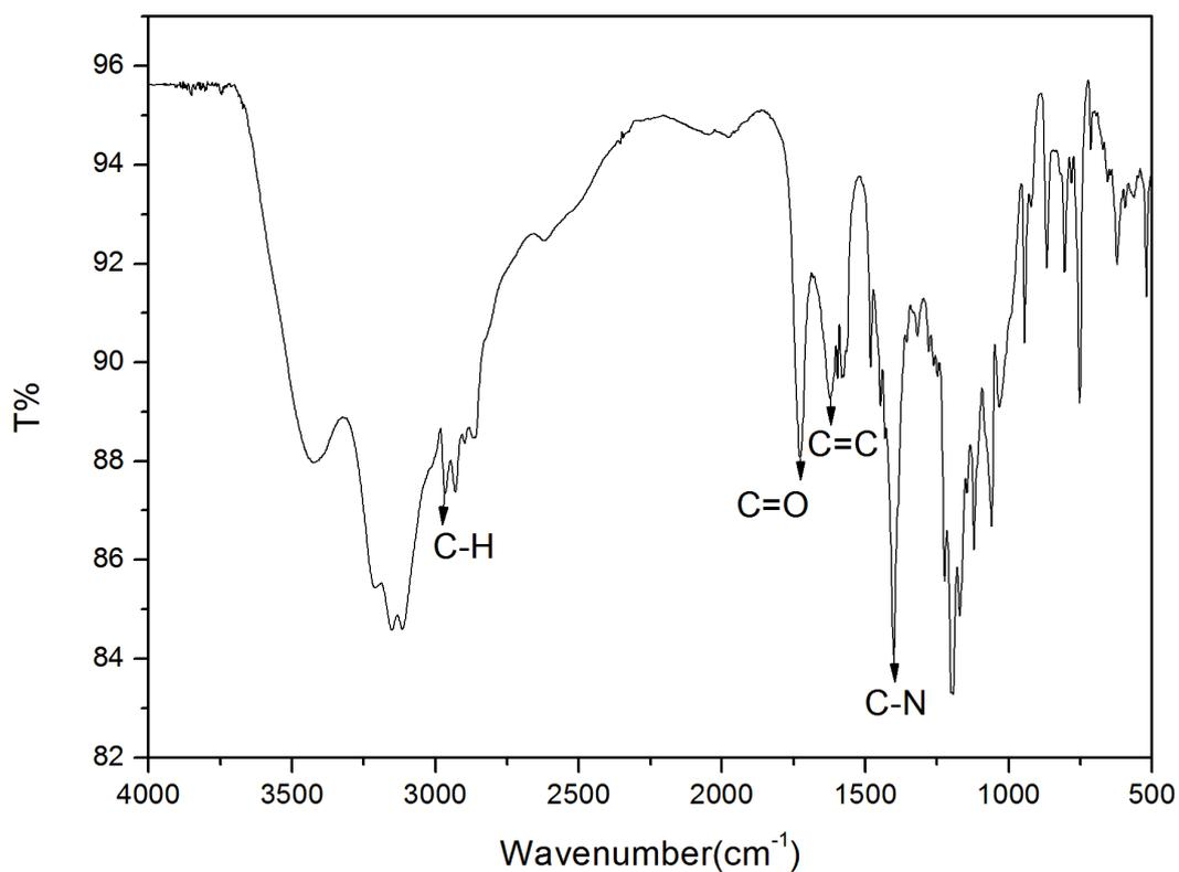
Figure S1. FT-IR spectrum of EC-g2
