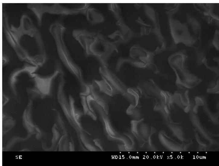
Figure S4. SEM images of ethyl cellulose blended 1-carboxymethyl-3-methylimidazolium gas separation membrane
