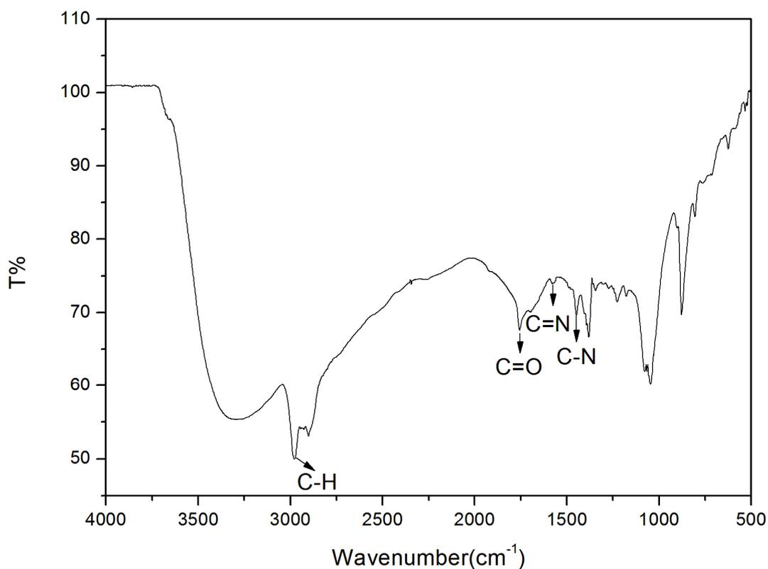
Figure S3. FT-IR spectrum of EC-g4
