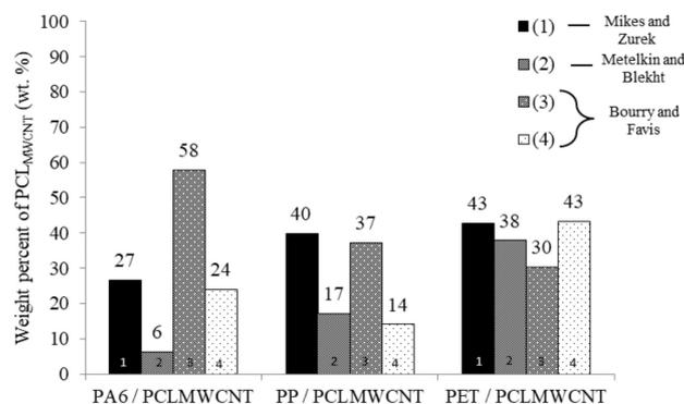
**Figure 2.** Results of co-continuity of models of Mikes and Zurek, Metelkin and Blekht, and Bourry and Favis for the blend PA6/PCL<sub>MWCNT</sub>, PP/PCL<sub>MWCNT</sub>, and PET/PCL<sub>MWCNT</sub> according to the weight percent of filled PCL with 1.5 wt.% of MWCNT (wt.%).
