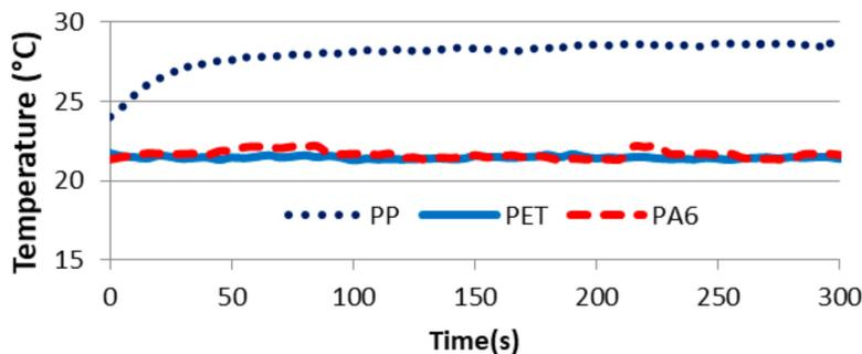
**Figure 7.** Comparison of the temperature ( $^{\circ}\text{C}$ ) increase according to the time (s) for the blends of PA6/PCL<sub>MWCNT</sub>, PP/PCL<sub>MWCNT</sub>, and PET/PCL<sub>MWCNT</sub>.
