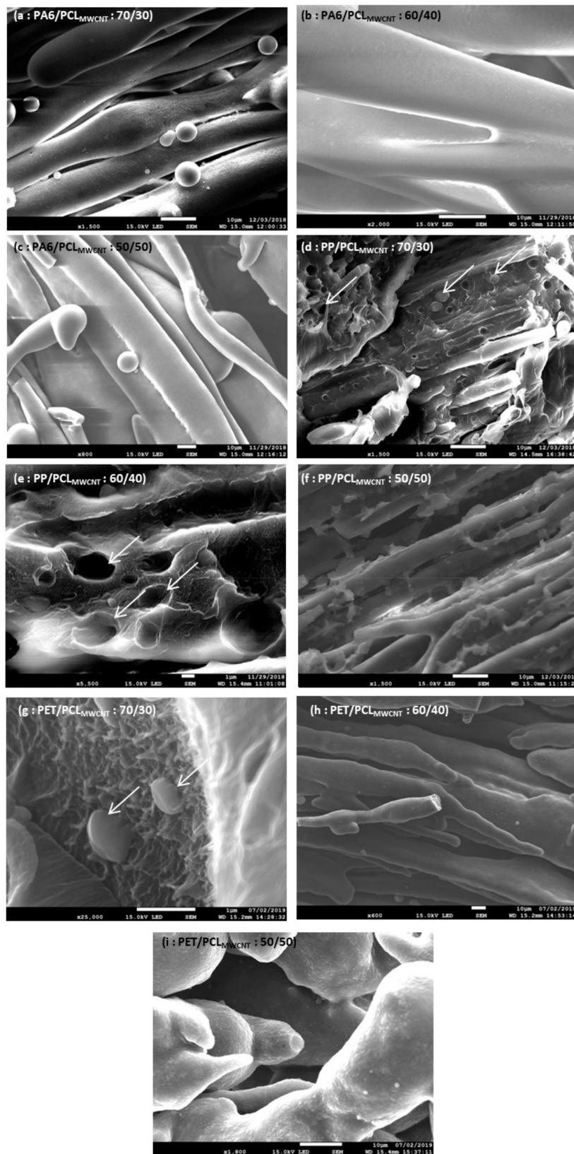
**Figure 4.** SEM images of PA6/PCL<sub>MW/CNT</sub> (a) 70/30, (b) 60/40, (c) 50/50; PP/PCL<sub>MW/CNT</sub> (d) 70/30, (e) 60/40, (f) 50/50; and PET/PCL<sub>MW/CNT</sub> (g) 70/30, (h) 60/40, (i) 50/50 after phase extraction.
