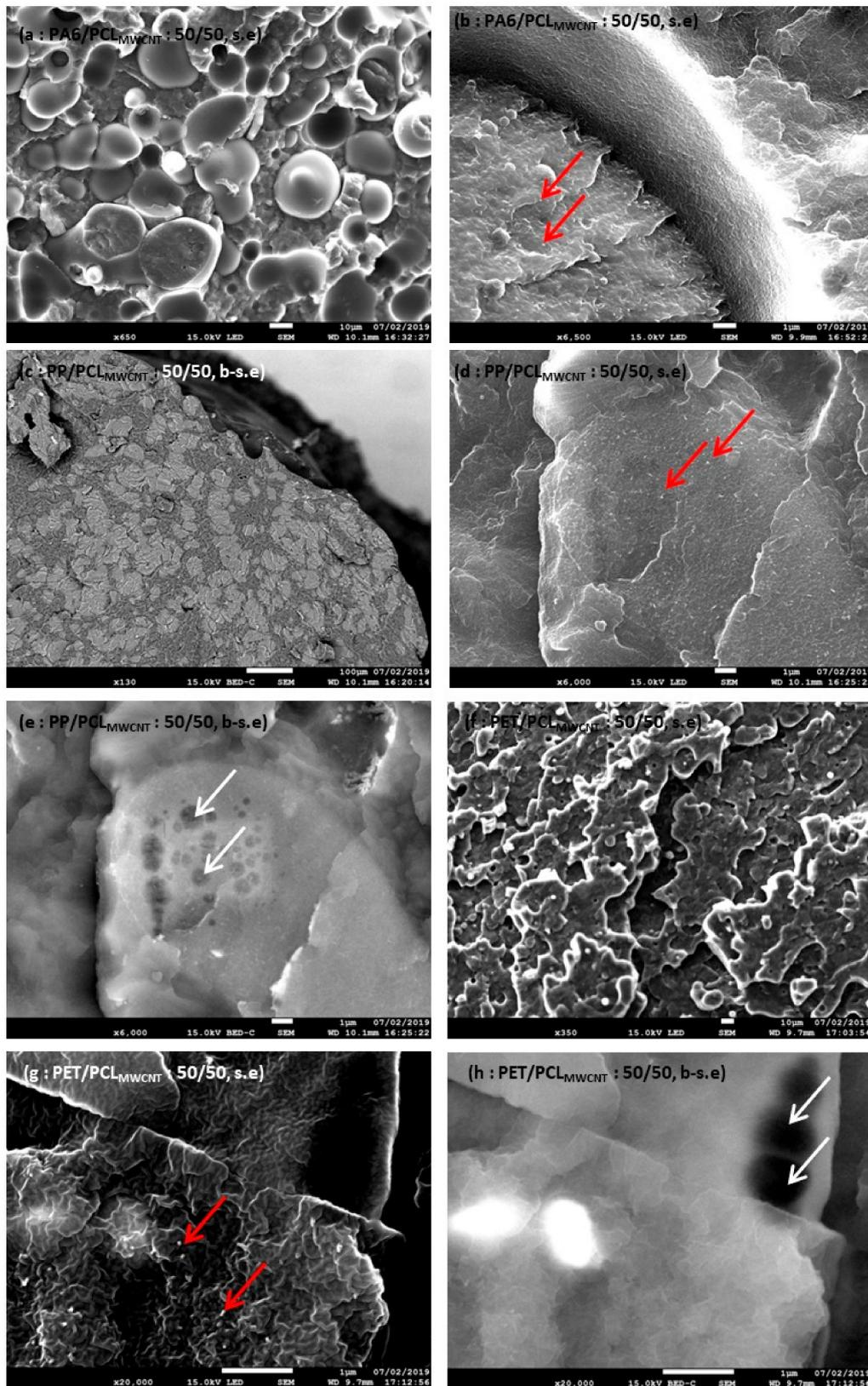
**Figure 5.** SEM images of PA6/PCL<sub>MWCNT</sub> 50/50 (a,b); PP/PCL<sub>MWCNT</sub> 50/50 (c–e); and PET/PCL<sub>MWCNT</sub> 50/50 (f–h).
