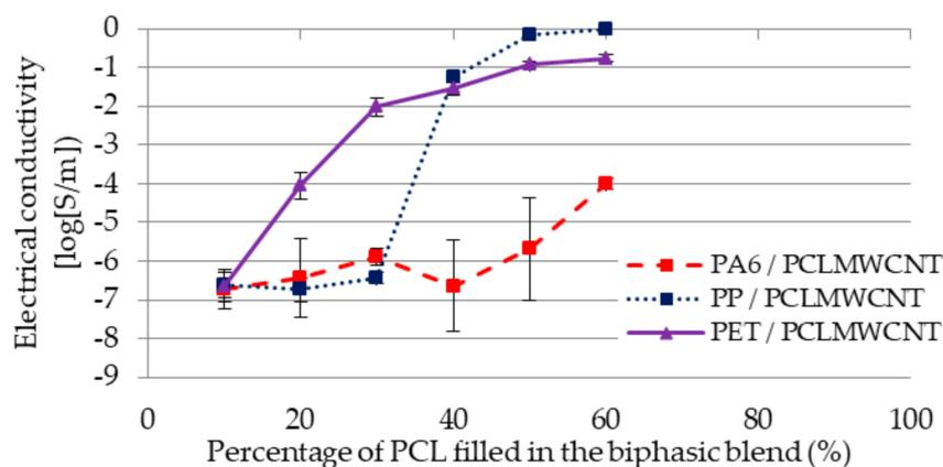
**Figure 6.** Comparison of the electrical conductivity ( $\log[S/m]$ ) according to the percentage of PCL<sub>MWCNT</sub> (wt.%) for the blends of PA6/PCL<sub>MWCNT</sub>, PP/PCL<sub>MWCNT</sub>, and PET/PCL<sub>MWCNT</sub>.
