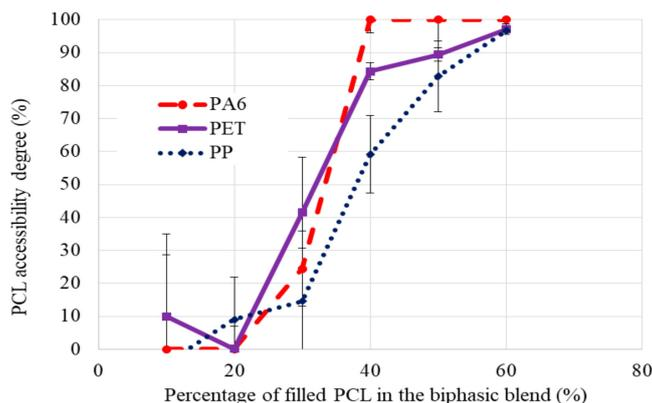
**Figure 3.** Comparison of percentage of filled PCL with 1.5 wt.% of MWCNT (wt.%) in PA6/PCL<sub>MWCNT</sub>, PP/PCL<sub>MWCNT</sub>, and PET/PCL<sub>MWCNT</sub> according to the PCL accessibility degree (%).
