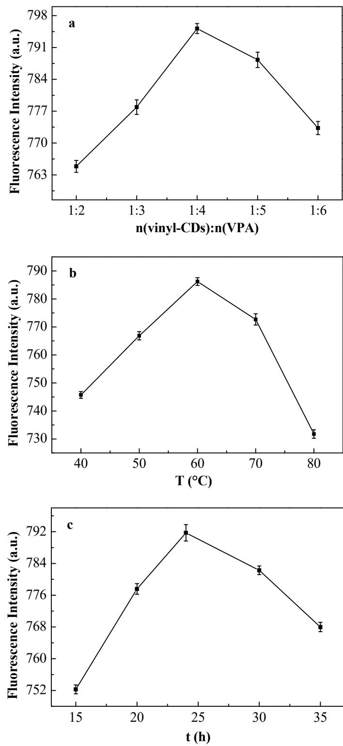
**Figure S6.** The effects of molar ratio (a), reaction temperature (b), and reaction time (c) values of reactants on the stability of CDs@VPA synthesized.
