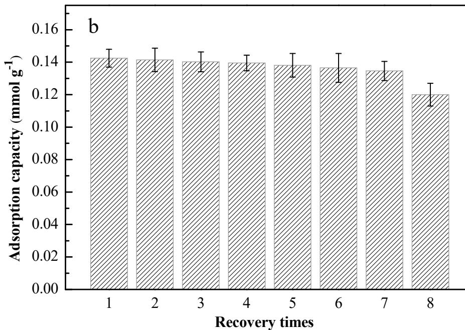
**Figure S3.** Selective recognition curves of MMIPs and MNIPs at 308 K (a); the recycling times of MMIPs' adsorption/desorption to triazophos (b). MMIPs means magnetic molecularly-imprinted polymeric microspheres prepared with triazophos as a template, while MNIPs are prepared without a template.
