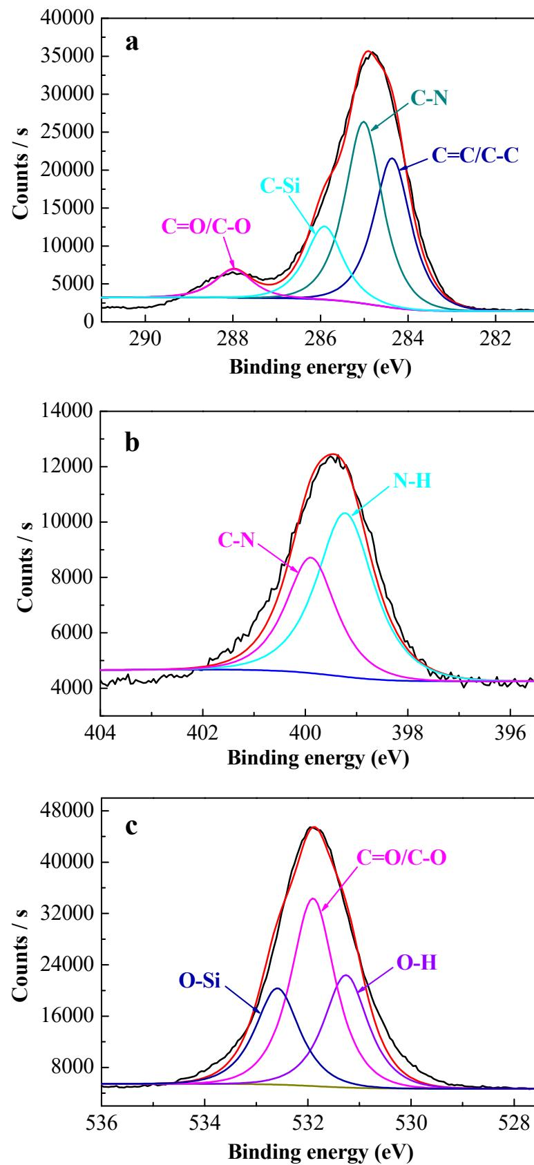
**Figure S8.** High resolution XPS spectra of C 1s (a), N 1s (b), and O 1s (c) of CDs.
