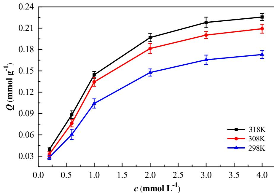
**Figure S2.** Adsorption thermodynamics curves of MMIPs.
