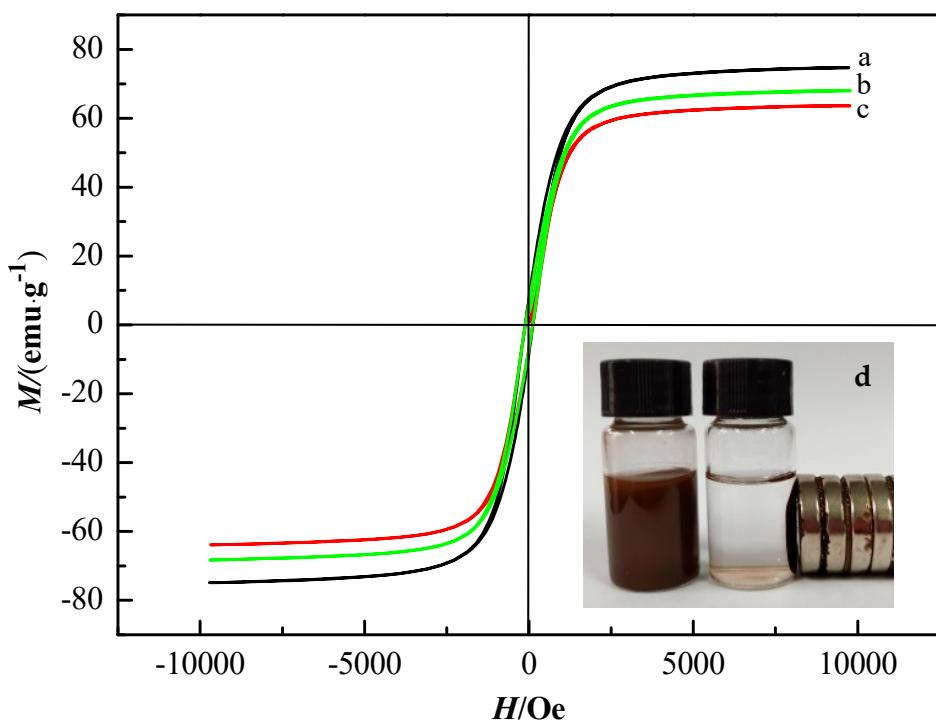
**Figure S4.** The magnetization curves of Fe<sub>3</sub>O<sub>4</sub> (a), Fe<sub>3</sub>O<sub>4</sub>@mSiO<sub>2</sub> (b), MMIPs (c), and magnetically controlled separation of MMIPs under the effect of magnets (d).
