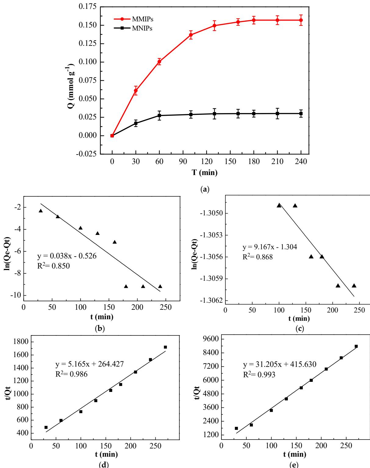
**Figure S1.** The adsorption kinetics curves of MMIPs and MNIPs at 308 K (a); First-order dynamics simulation of MMIPs (b) and MNIPs (c). Second-order dynamics simulation of MMIPs (d) and MNIPs (e), which depend on Equations (5) and (6), respectively.
