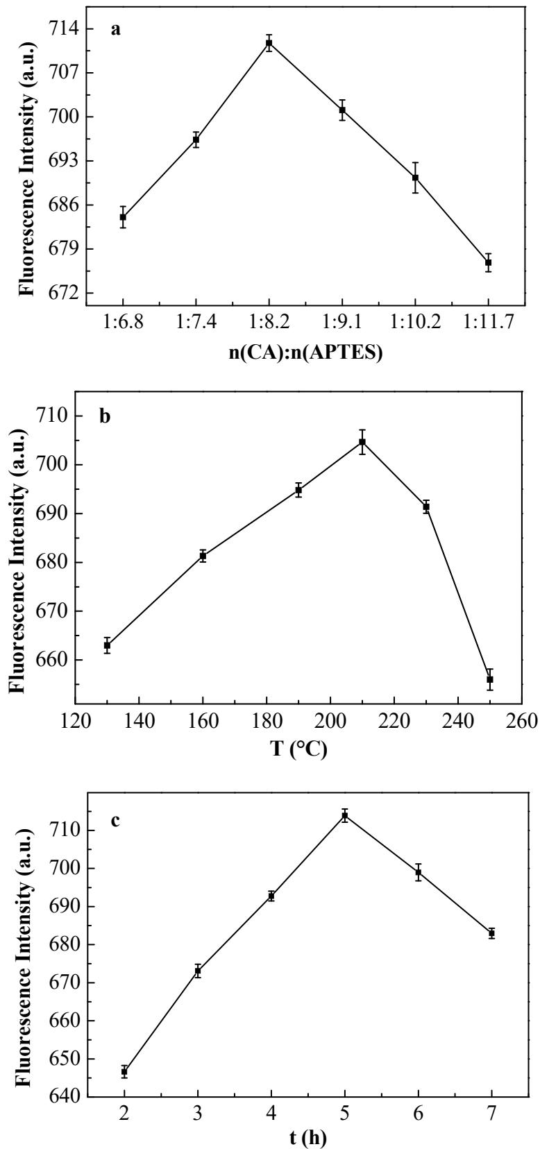
**Figure S5.** The effects of molar ratios (a), reaction temperatures (b), and the reaction times (c) of reactants on the stability of CDs synthesized.
