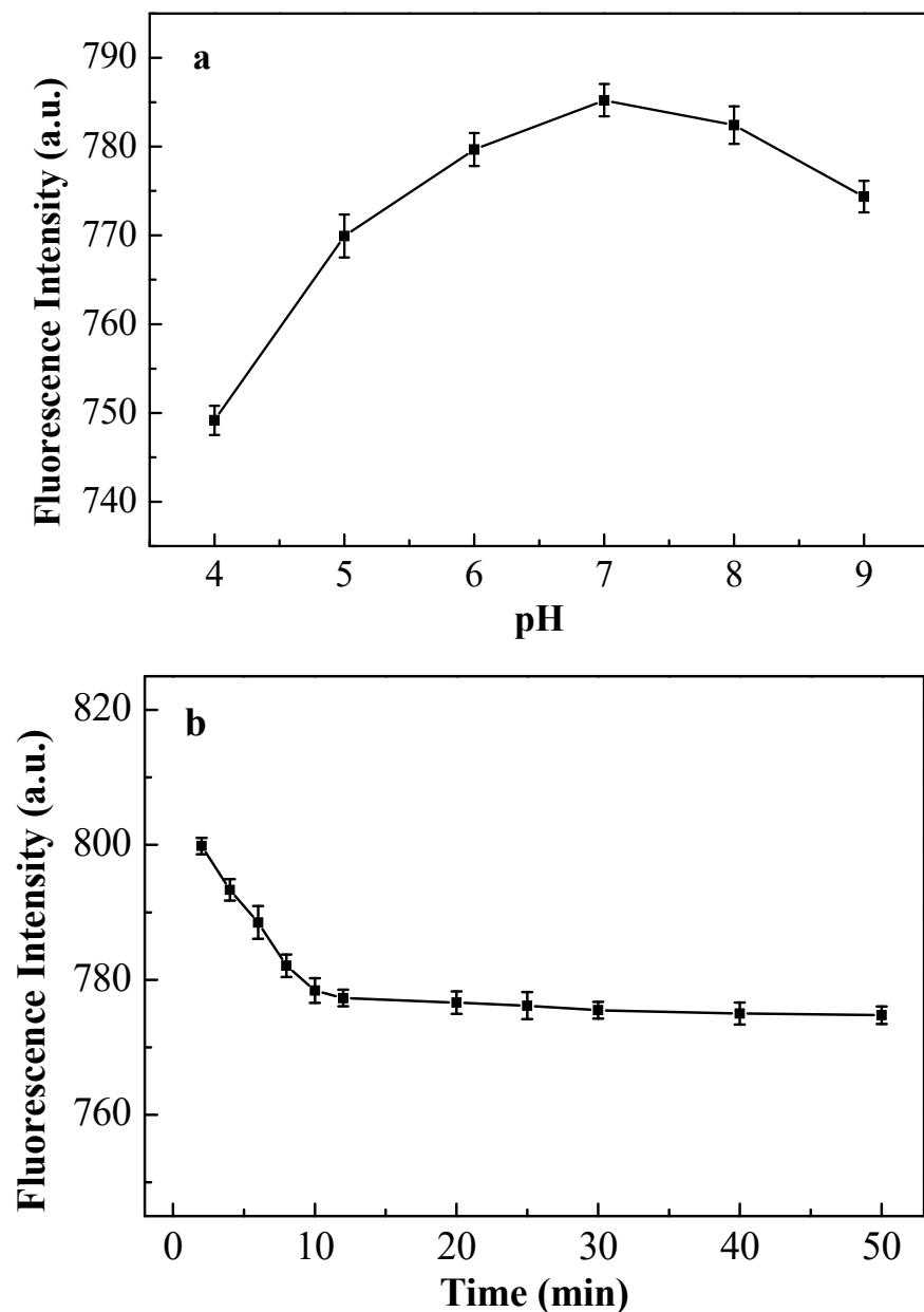
**Figure S7.** The effects of pH (a) and incubation time (b) on the stability of the CDs@VPA detected.
