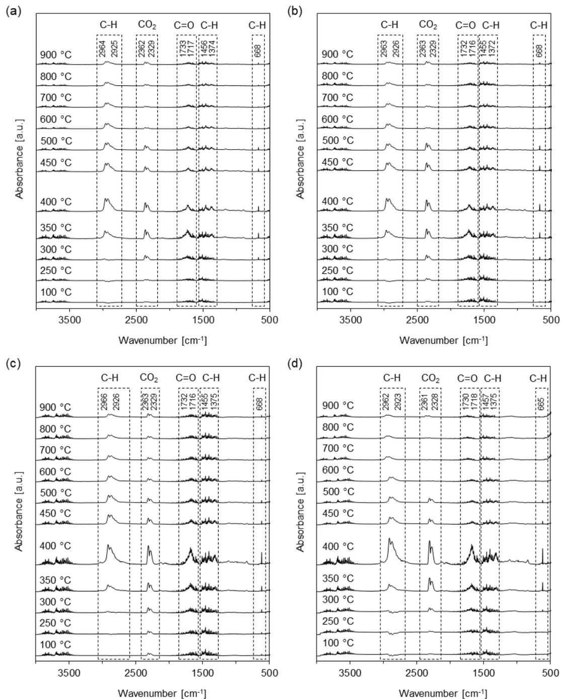
**Figure 4.** 2D thermogravimetry-Fourier transform infrared spectrometry (TG-FTIR) spectra of pyrolysis products of (a) neat PP, (b) PP/1%S4SQ-H, (c) PP/1%S4SQ-8 and (d) PP/1%S4SQ-18 at various temperatures.
