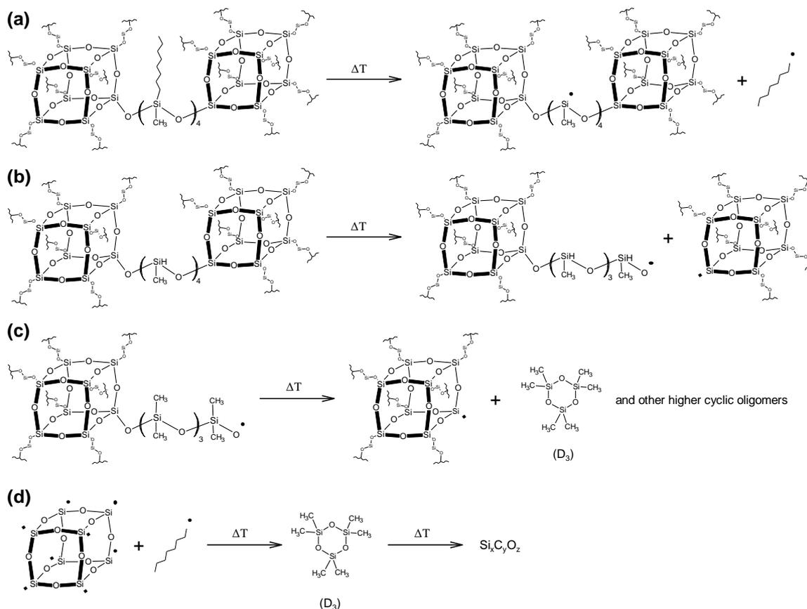
**Scheme 1.** A possible mechanism for the thermal degradation of siloxane-silsesquioxane resins followed by (a) split-off of the alkyl substituents from the siloxane groups, (b) detachment of the siloxane chains from the silsesquioxane cages, (c) split of the siloxane chains from the resin structure and (d) thermal decomposition of the silsesquioxane cages to small cyclic oligomers and then to the ceramic  $\text{Si}_x\text{C}_y\text{O}_z$  structure.
