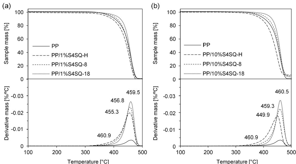
**Figure 2.** TG/DTG curves of neat PP as well as (a) PP/1%S4SQ and (b) PP/10%S4SQ composites (under nitrogen atmosphere).
