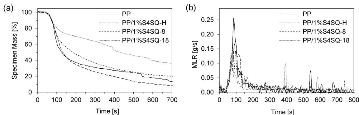
**Figure 8.** Mass curves during combustion for neat PP and PP/S4SQ composites: (a) sample mass (normalized on initial weight) and (b) mass loss rate (MLR).
