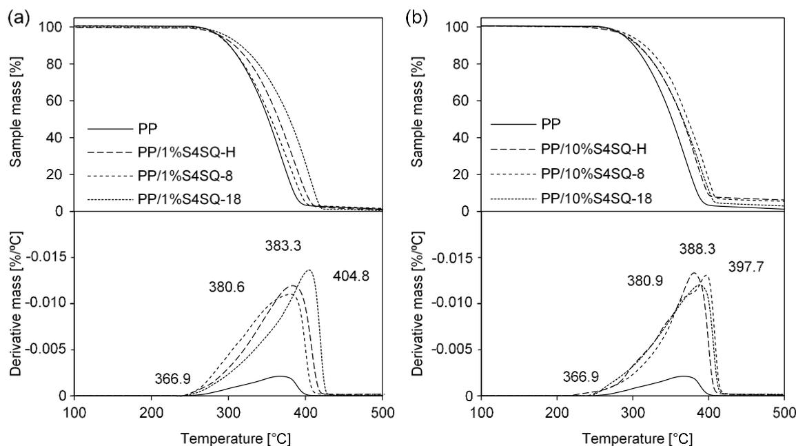
**Figure 3.** TG/DTG curves of neat PP as well as (a) PP/1%S4SQ and (b) PP/10%S4SQ composites (in air atmosphere).
