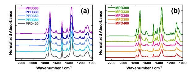
Figure S1. Mid-IR-ATR spectra of (a) PPD-PI and (b) MPD-PI films cured at different temperatures.
