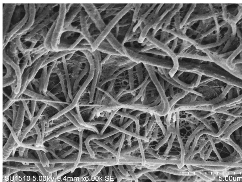
**Figure 5.** SEM images for BC/CA-ENM hybrid mats cross-sectional morphology.
