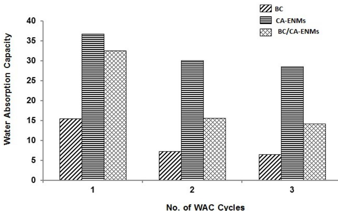
**Figure 9.** Percentage of the water absorbed in the BC films, CA-ENMs, and BC/CA-ENM hybrid mats after three wetting-drying cycles.
