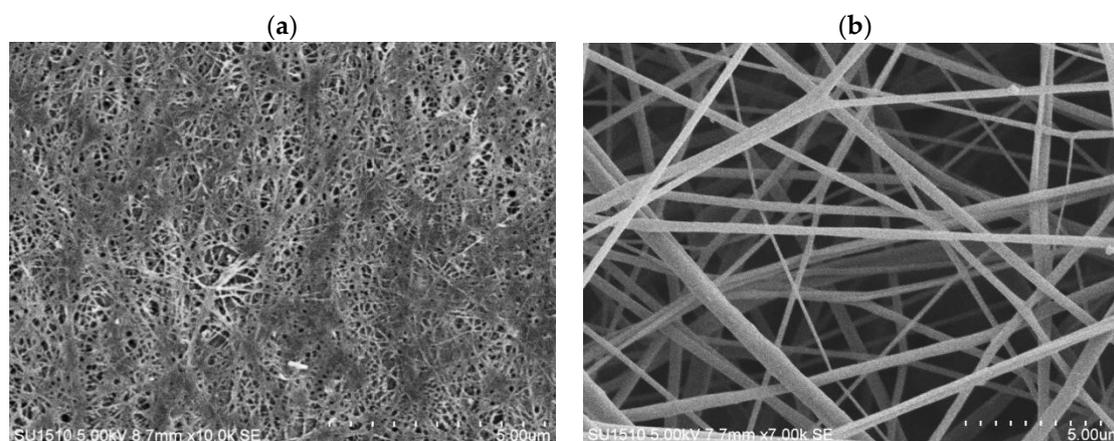
**Figure 2.** (a,b) SEM images for BC film (a) and CA-ENMs (b) sample surface morphology.
