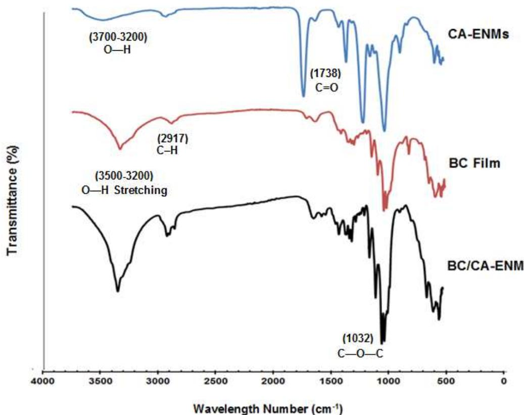
Figure 6. FTIR analysis graphs for BC films, CA-ENMs, and BC/CA-ENM hybrid mat samples.
