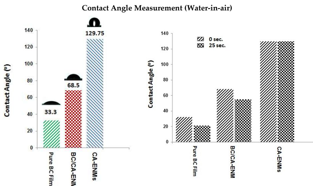
**Figure 8.** Contact angle measurement for pure BC films, BC/CA-ENM hybrid mats, and CA-ENMs.
