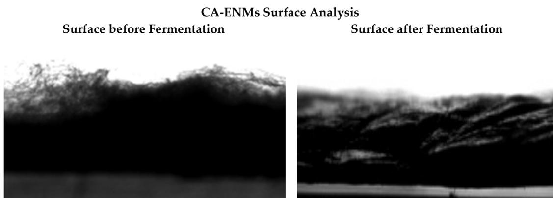
**Figure 4.** Photographs of CA-ENM surfaces before fermentation (**left**) and after seven days of fermentation (**right**).
