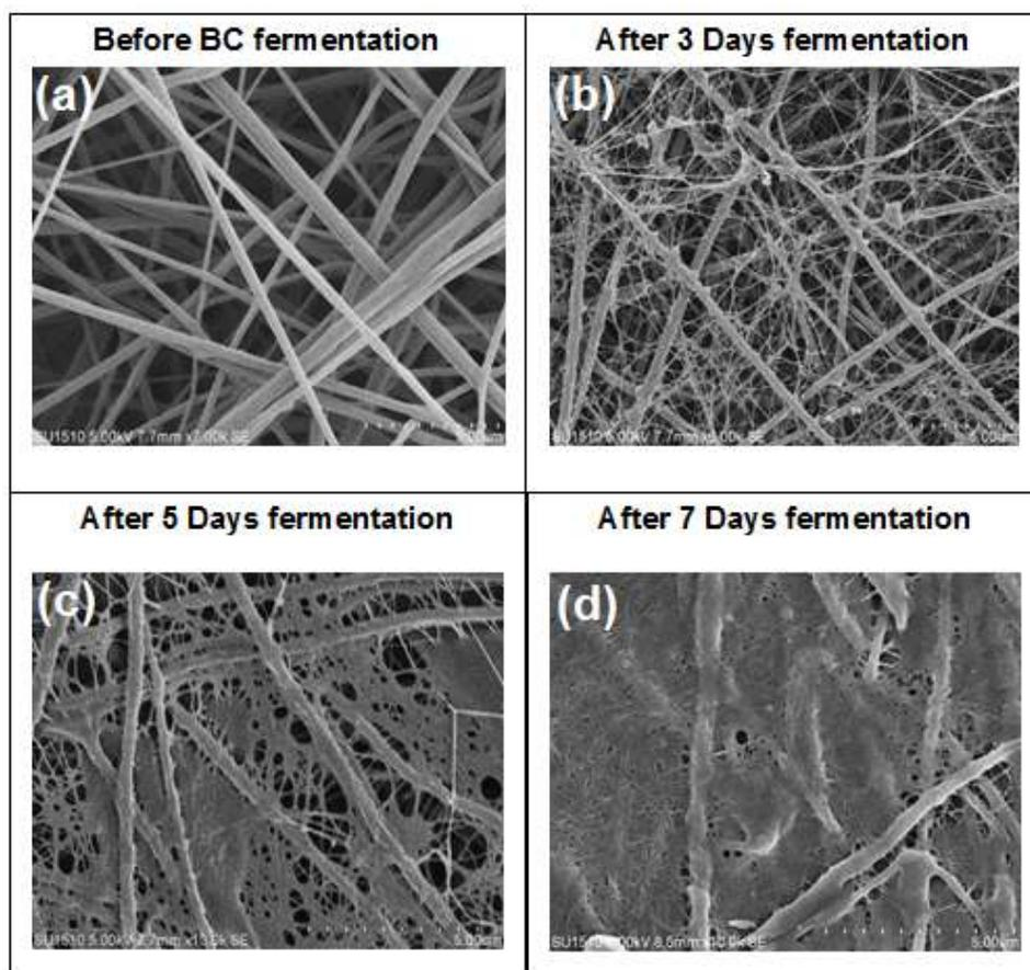
**Figure 3.** SEM images for BC/CA-ENM hybrid mats; surface morphology: (a) before fermentation; (b) after three days of fermentation; (c) after five days; and (d) after seven days.
