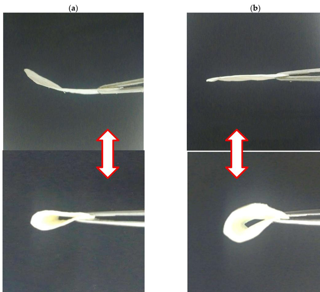
**Figure 10.** Flexibility analysis of Pure BC film (a) and as-prepared BC/CA-ENM hybrid mat (b) samples.
