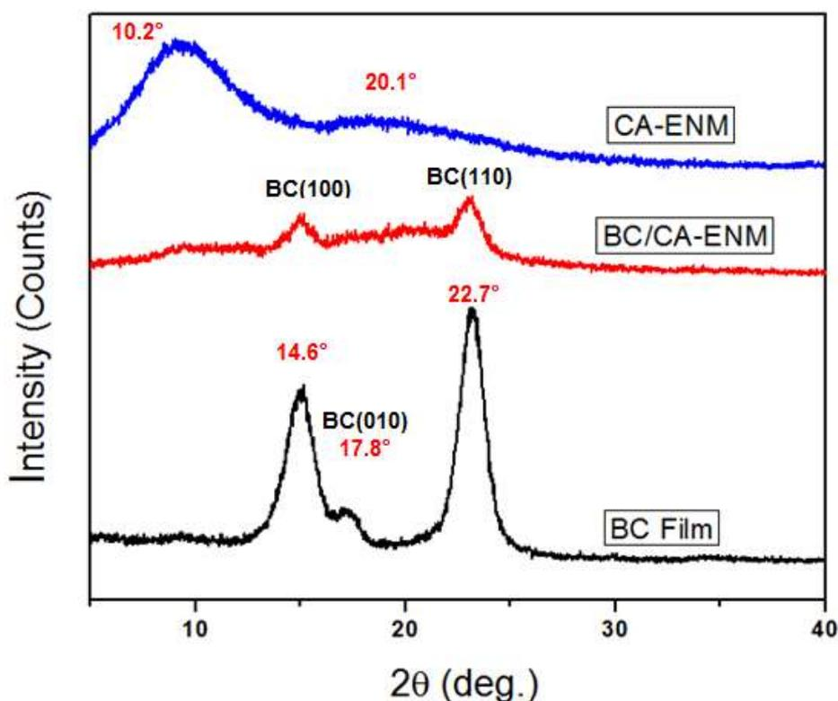
**Figure 7.** XRD diffractograms of BC films, CA-ENMs, and BC/CA-ENM hybrid mat samples.
