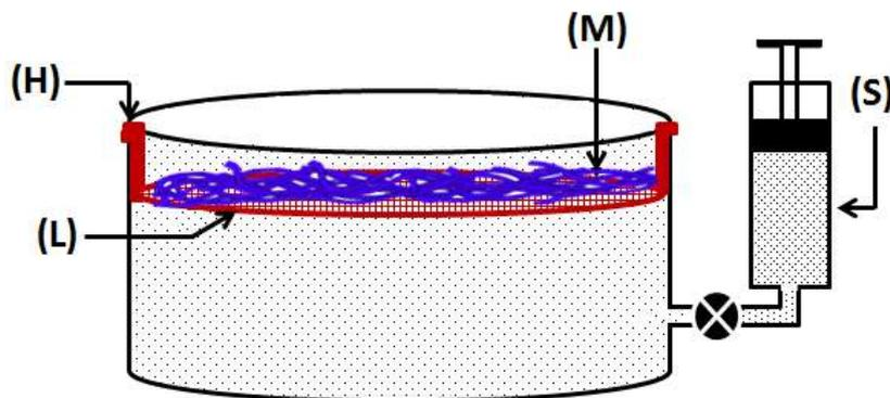
**Figure 1.** Schematic diagram of customized apparatus used for fabrication of in situ self-assembled bacterial cellulose-electrospun nanofiber hybrid mats.
