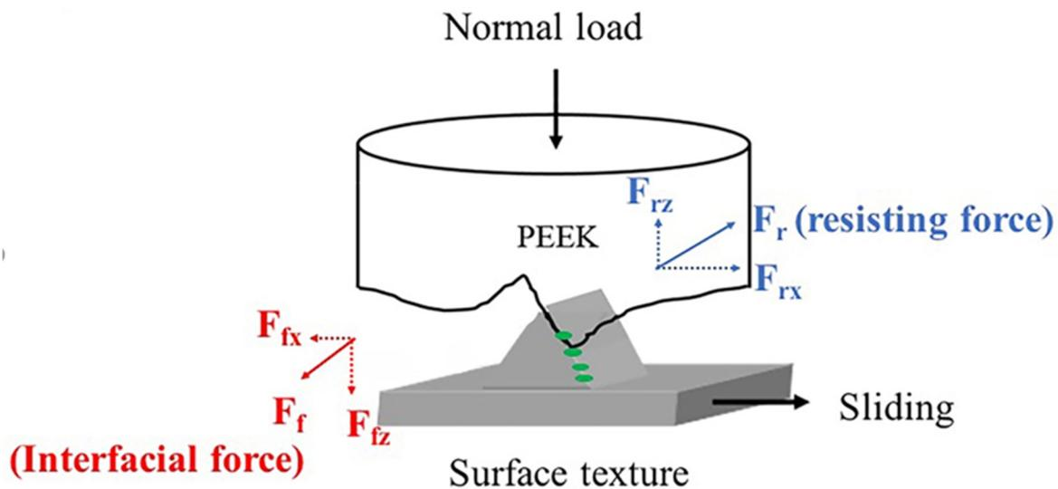
**Figure 4.** Mechanical analysis of the resisting force and interfacial friction for the surface feature sliding over PEEK process.  $F_{rz}$  is upward direction of the resisting force;  $F_{rx}$  is horizontal direction of the resisting force;  $F_{fz}$  means downward direction of the interfacial friction;  $F_{fx}$  is horizontal direction of the interfacial friction. Green circles represent the testing components such as HSA, IgG, or DPPC.
