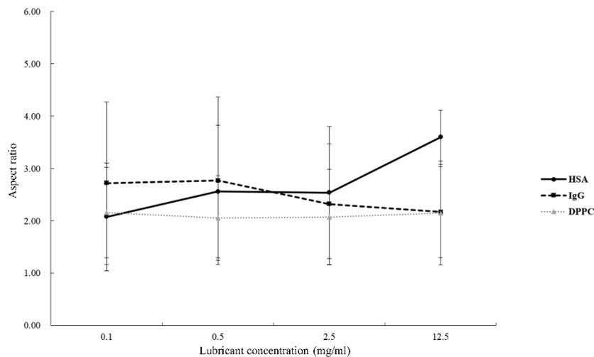
**Figure 3.** Aspect ratio of PEEK wear particles under the lubrication of HSA, IgG or DPPC solution. Plots of aspect ratio and the wear rate in different concentrations of HSA, IgG or DPPC solution.
