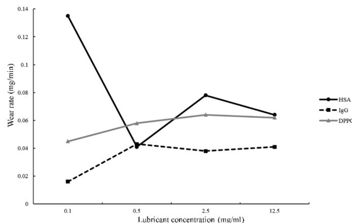
**Figure 5.** Wear rate of PEEK wear particles under the lubrication of HSA, IgG, or DPPC solution. Plots of aspect ratio and the wear rate in different concentrations of HSA, IgG or DPPC solution.
