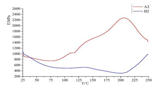
Figure 21. Comparative themomechanical analysis (TMA) traces of curing of A2 and B2 NIPU resins on wood.
