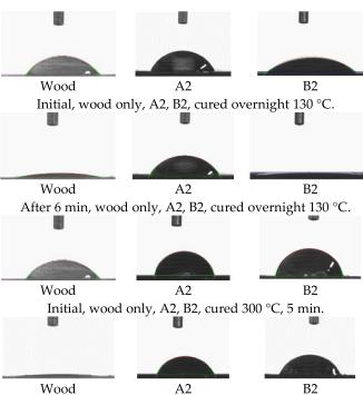
After 7 min, wood only, A2, B2, cured 300 °C, 5 min.
