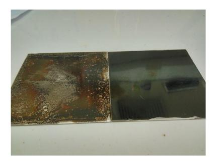
**Figure 22.** B2 (**left**) and A2 (**right**) NIPU resin surface coatings on stainless steel plates after curing at 300 °C for 3 min.
