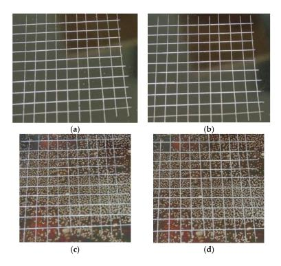
**Figure 23.** Cross-cut test according to NF EN ISO 2409 of glucose-based and sucrose-based surface coatings on stainless steel cured for 3 min at 300  $^{\circ}$ C. (a) A2 before washing in hot water; (b) A2 after washing in hot water; (c) B2 before washing in hot water; and (d) B2 after washing in hot water.
