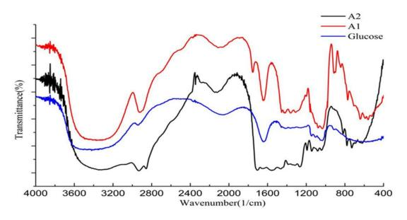
Figure 18. FTIR spectra of glucose, carbonated glucose A1, and glucose-based A2 NIPU resin.
