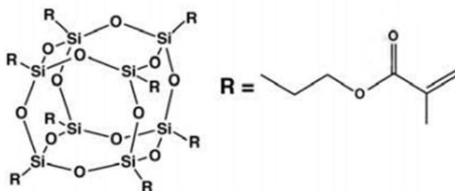
**Figure 1.** The molecule structure of methacryl polyhedral oligomeric silsesquioxane (POSS).
