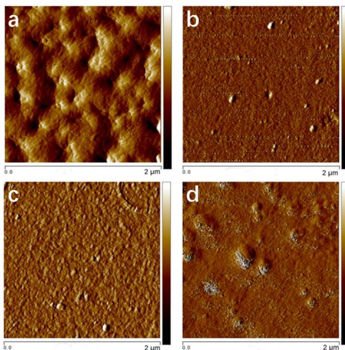
**Figure 2.** The atomic force microscopy (AFM) images of the structure of composite resins with different POSS additions: (a) P00, (b) P02, (c) P05, (d) P10.
