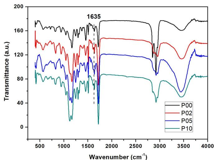
Figure 3. FTIR spectra of composite resins with different POSS additions.
