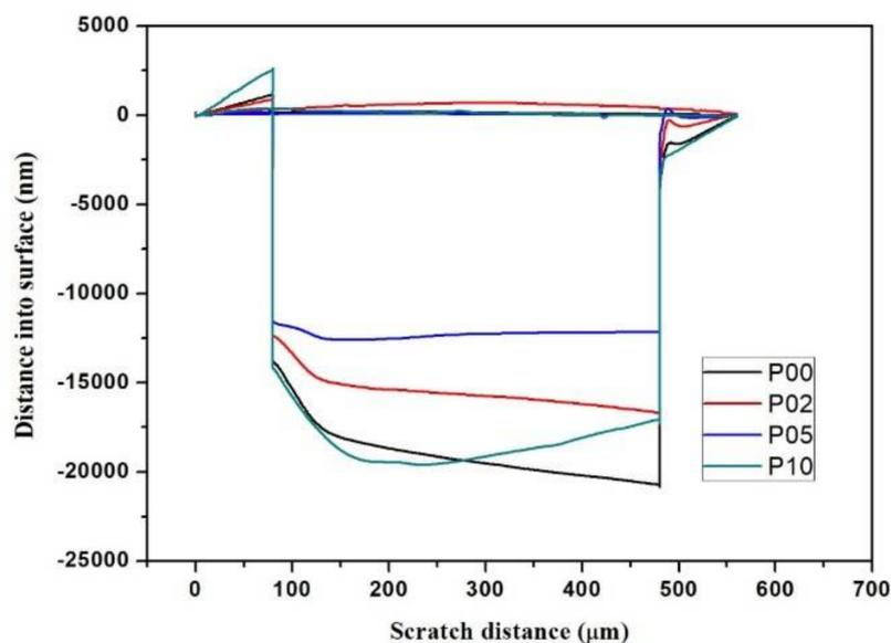
**Figure 5.** Influence of composite resins with different POSS additions on the scratch profiles.
