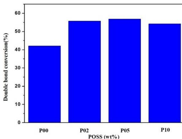
Figure 4. Double bond conversion of composite resins with different POSS additions.
