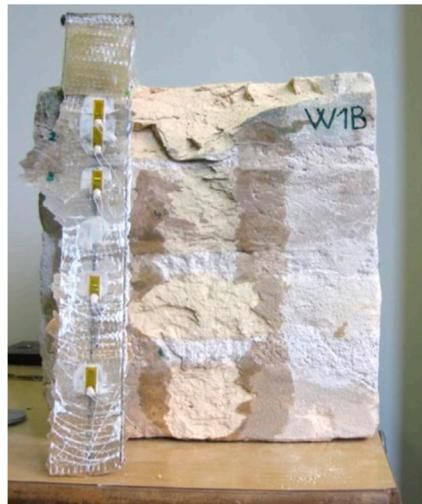
**Figure 1.** Typical delamination failure of GFRP strip-to-historic-brickwork joint [3]. Reprinted from *Composite Structures*, 140, Capozucca R., Ricci V., Bond of GFRP strips on modern and historic brickwork masonry, 540–555, Copyright (2016), with permission from Elsevier.
