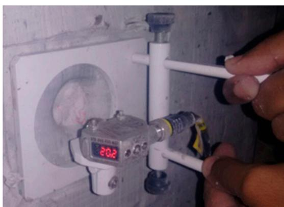
**Figure 4.** Depth of indentation in the clay witness measured with laser sensor caliper.
