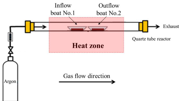
Figure S2. Schematic of the furnace system.
