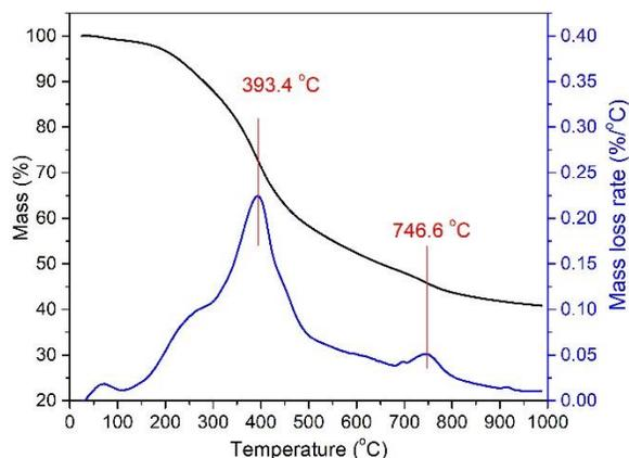
Figure S1. Thermogravimetric analysis of KL/Fe showing TG and DTG curves.
