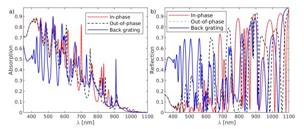
**Figure 7.** (a) simulated spectral response of the active layer's optical absorption in structures with only a periodic back grating (solid blue line), an out-of-phase double grating (black dashed line) and an in-phase double grating (red dash-dotted line); (b) simulated spectral response of the reflected power for all mentioned structures.
