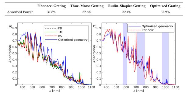
**Figure 11.** (a) simulated spectral response of the active layer's optical absorption in structures with double gratings, such as the optimized semiperiodic double grating, the double grating based on Fibonacci (FB), Thue–Morse (TM) and Rudin–Shapiro (RS) sequences; (b) comparison between the optimized semiperiodic double grating and the fully periodic double grating.
