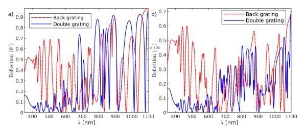
**Figure 4.** simulated spectral response of the reflected power in structures with a periodic back grating (red dash-dotted line) and with a periodic double grating (blue line) at (**a**) normal incidence and at (**b**)  $\frac{\pi}{8}$  tilted incidence.
