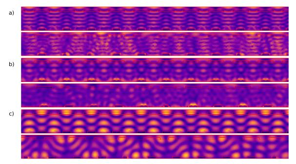
**Figure 12.** simulated electric field distributions at different operating wavelengths of (**a**) 583 nm; (**b**) 764 nm; and (**c**) 1014 nm highlighted in Figure 11, for solar cell topologies with a periodic double grating (top) and an optimized semiperiodic double grating (bottom).
