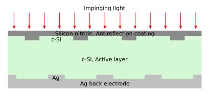
Figure 1. schematic of the solar cell structure.
