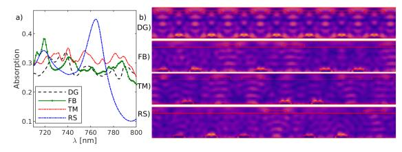
**Figure 9.** (a) simulated spectral response of the active layer's optical absorption in structures with a periodic double grating (DG) along with double gratings based on Fibonacci (FB), Thue–Morse (TM) and Rudin–Shapiro (RS) sequences; (b) simulated electric field distributions at an operating wavelength of 764 nm for all of the mentioned structures.
