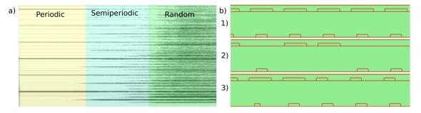
**Figure 8.** (a) schematic illustration of semiperiodicity; (b) geometry of a periodic (1), a Thue–Morse semiperiodic (2) and an optimized semiperiodic double grating (3).
