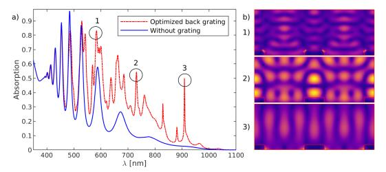
**Figure 2.** (a) simulated spectral response of the active layer's optical absorption in structures without periodic back grating (solid blue line) and with optimized periodic back grating (red dash-dotted line); (b) simulated electric field distributions at the operating wavelengths as labelled in the graph (a).
