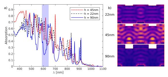
**Figure 5.** (a) simulated spectral response of the active layer's optical absorption in structures with a periodic double grating and tooth heights of 90 nm (solid blue line), 45 nm (red dash-dotted line) and 22 nm (black dashed line); (b) simulated electric field distributions at the operating wavelength of 620 nm highlighted in the graph (a), for all mentioned tooth heights.
