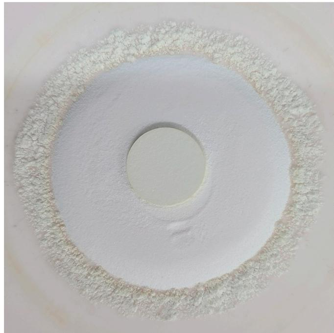
**Figure 1.** Image of sample in the setup after sintering without contact with the bed powder.
