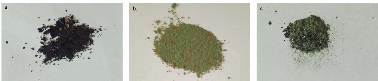
Figure S1 Photos of samples without adding sodium fluoride and 1 day's synthesis (a), with a F/V molar ratio of 0.1 in starting mixture and 1 day's synthesis (b) and 3 days' synthesis (c).
