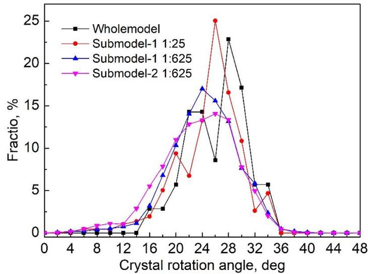
Figure 5. Distribution of crystal rotation angles in Grain A.
