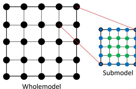
Figure 1. Submodel modelling method.
