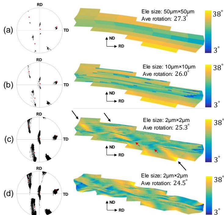
**Figure 4.** (1 1 1) pole figures and distribution of crystal rotation angles of Grain A in the (a) Wholemodel, (b) Submodel-1 1:25, (c) Submodel-1 1:625 and (d) Submodel-2 1:625. The initial orientations are shown in red, and final orientations in black. Black arrows indicate grain-scale shear bands, while micro-scale shear bands are marked by red arrows.
