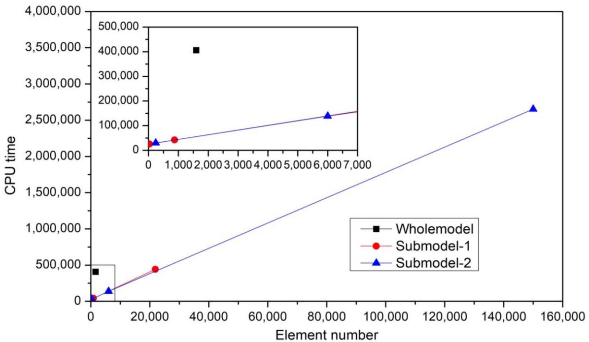
Figure 6. Relation between element number and CPU time in seconds.
