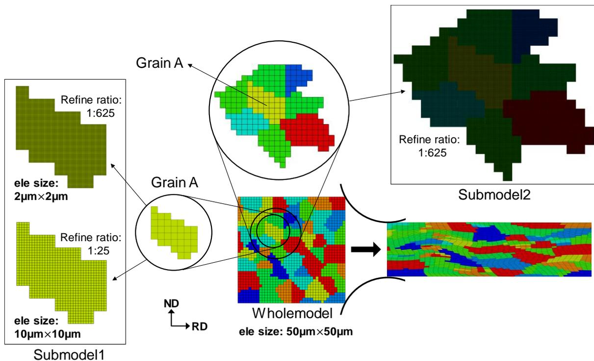
**Figure 2.** Mesh resolution of selected grains in Submodel and Wholemodel.
