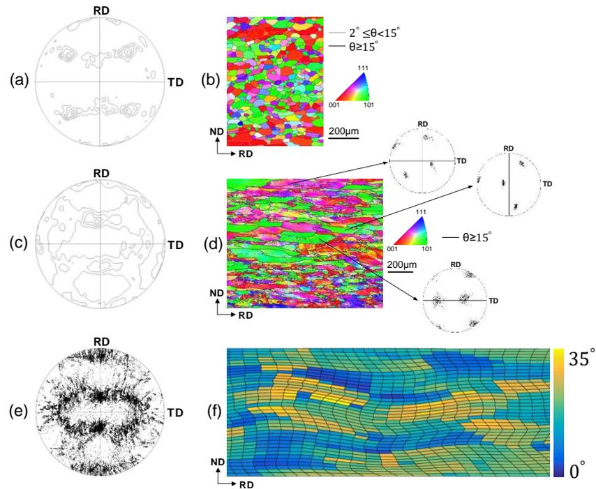
**Figure 3.** (1 1 1) pole figures of the global texture (a) before rolling, (c) after rolling and (e) in the Wholemodel. IPF EBSD maps (b) before rolling and (d) after rolling, and (f) distribution of crystal rotation angles in the Wholemodel.
