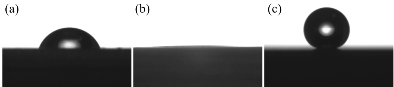
Figure 2. The contact angles of the three surfaces: (a) the original sample, (b) the LT sample, (c) LT and HT samples.
