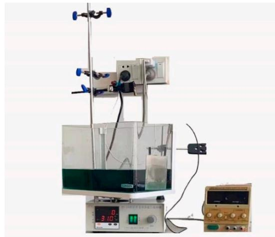
**Figure 1.** Electroplating Operation Console.
