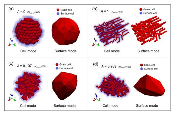
**Figure 2.** Schematic view of (**a**) volume-equivalent-sphere, (**b**) volume-equivalent-chain, and (**c**,**d**) two grains with volume of 500.
