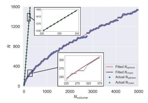
**Figure 3.** Relationships between surface cell number of volume-equivalent-sphere (red curve and blue dots), volume-equivalent-chain (black curve and green dots), and their corresponding grain volume number.
