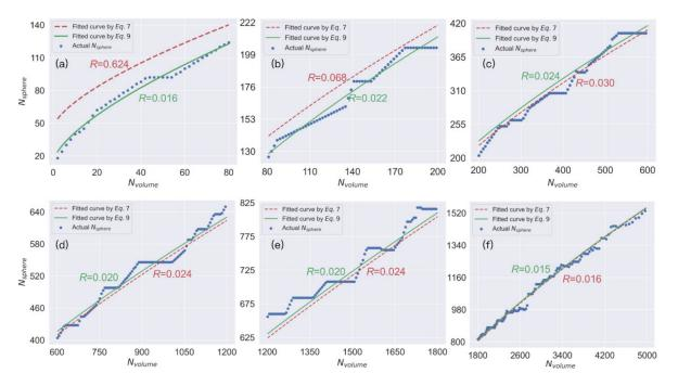
**Figure 4.** Comparison of fitting effect between Equation (9) and Equation (7) with volume number within a range of (**a**) 1~79, (**b**) 80~199, (**c**) 200~599, (**d**) 600~1199, (**e**) 1200~1799, and (**f**) 1800~5000.
