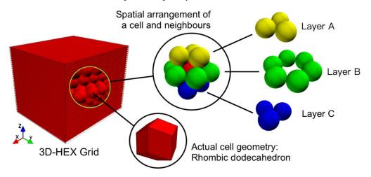
Figure 1. Schematic view of 3D-HEX grid and spatial arrangement of a cell and its neighbors.
