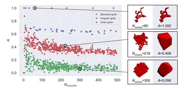
Figure 5. Distribution of shape factor of spherical grain, irregular grain, and chain grain.
