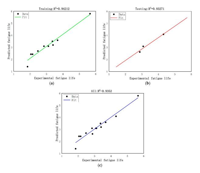
**Figure 5.** The regression plots for the model predicting fatigue life. (**a**) Training data. (**b**) Testing data. (**c**) All data.
