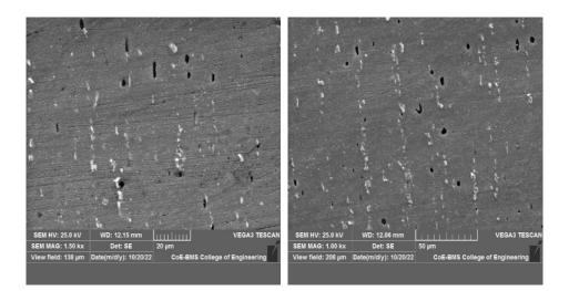
Figure 2. SEM images of FSPed AA7075 base metal.
