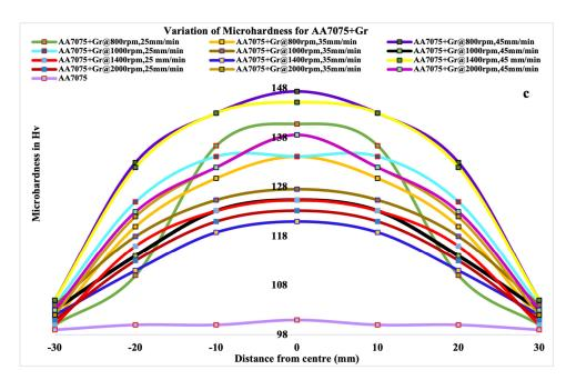
Figure 10. Micro-hardness profiles of AA7075 with (a) nB<sub>4</sub>C, (b) nTiO<sub>2</sub>, and (c) nGr FSPed.
