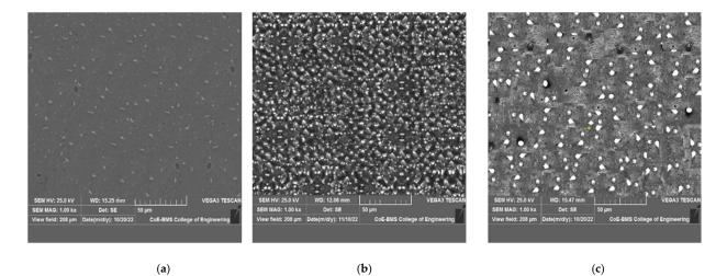
**Figure 4.** SEM images of a FSPed AA7075/ TiO<sub>2</sub> sample prepared at (**a**) 800 rpm and 35 mm/min, (**b**) 1000 rpm and 35 mm/min, and (**c**) 1000 rpm and 45 mm/min.
