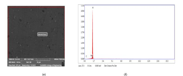
**Figure 3.** XRD analysis of (**a**) selected area and (**b**) EDAX of AA7075/n-B4C; (**c**) selected area and (**d**) EDAX of AA7075/n-TiO<sub>2</sub>; (**e**) selected area and (**f**) EDAX of AA7075/n-Gr.
