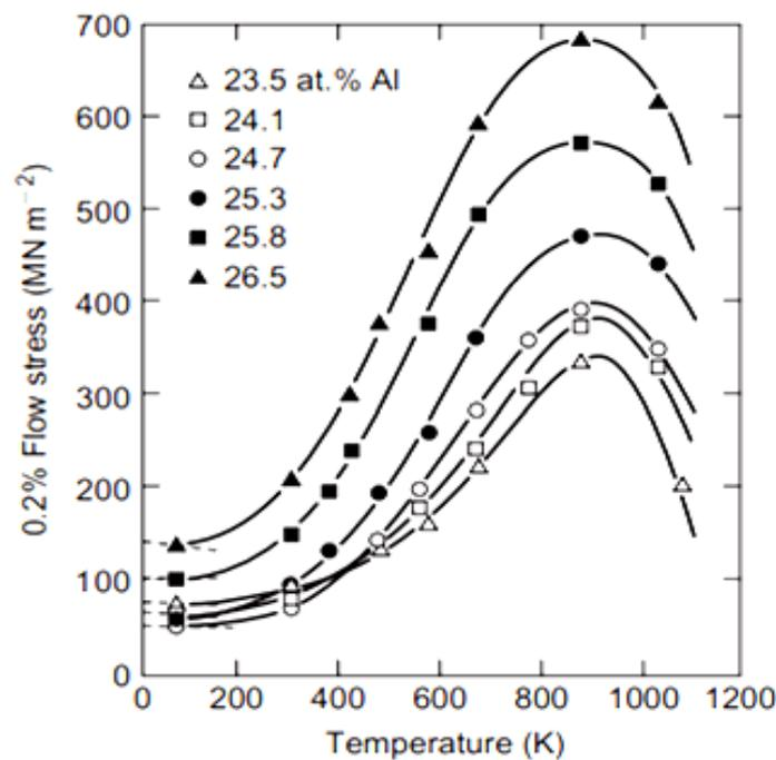
**Figure 5.** The influence of aluminum content on the temperature dependence of flow stress in Ni<sub>3</sub>Al [8]. Reproduced with permission from Elsevier.
