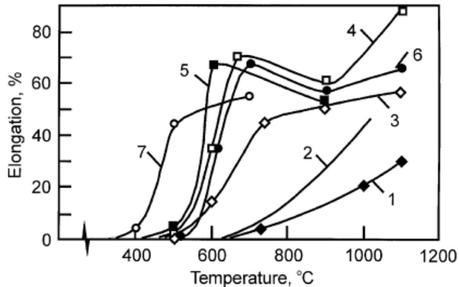
**Figure 10.** Elongation of NiAl alloys tested with 400–1200 °C. (1) casting of NiAl; (2) extruded NiAl; (3) NiAl(Mo); (4) NiAl(W); (5) NiAl(Fe); (6) NiAl(Cr); (7) NiAl (Co, B, La) [4]. Reproduced with permission from Elsevier.
