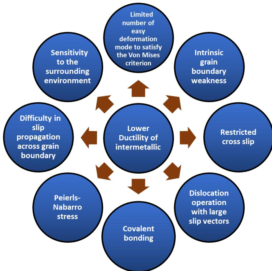
Figure 3. Factors that cause low ductility of intermetallics.
