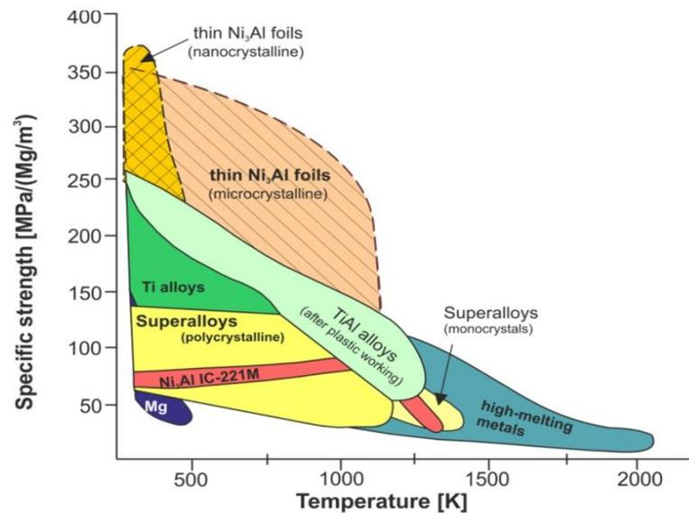
**Figure 13.** Temperature vs. specific strength for comparing Ni thin foils with other metal alloys [77]. Reused from MDPI under Creative Commons Attribution license.
