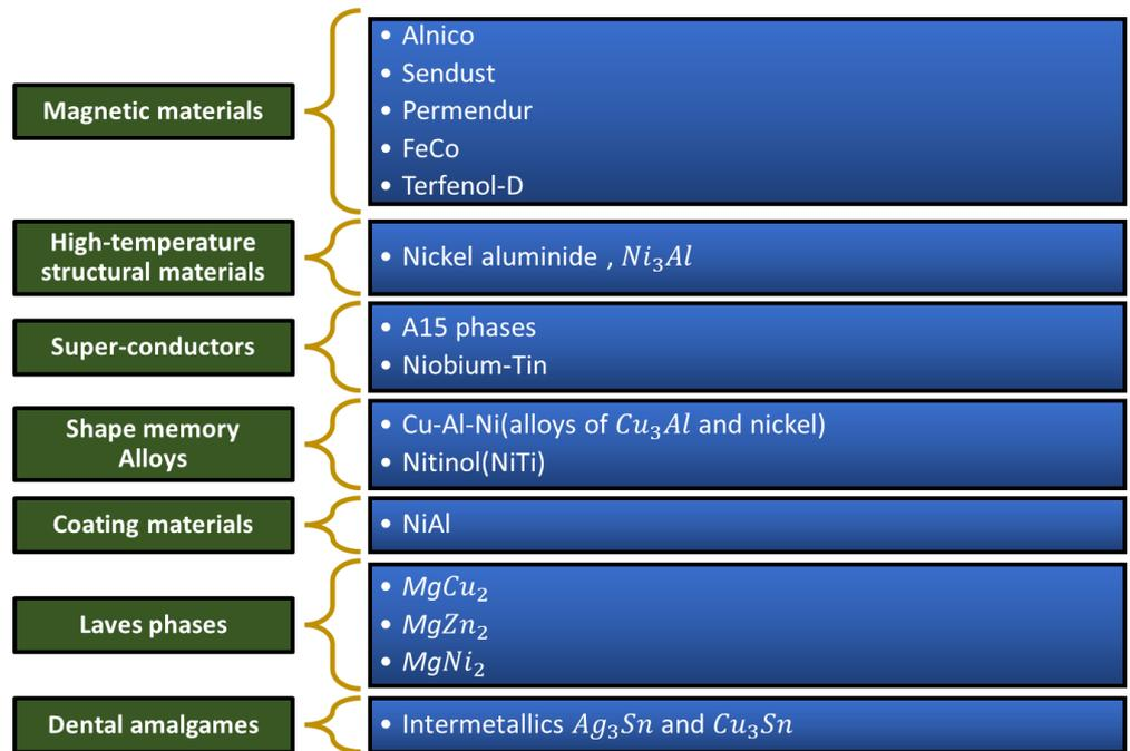
Figure 2. Classification of intermetallics based on properties.
