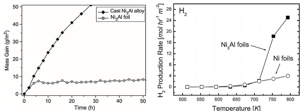
**Figure 14.** Comparison of production rates of H<sub>2</sub> in methanol decomposition of Ni<sub>3</sub>Al foils and Ni foils [77]. Reused from MDPI under Creative Commons Attribution license.
