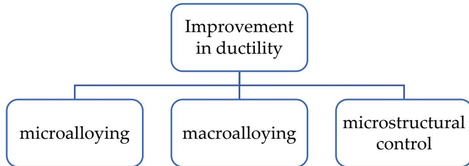
Figure 6. Different methods for improving ductility of NiAl.
