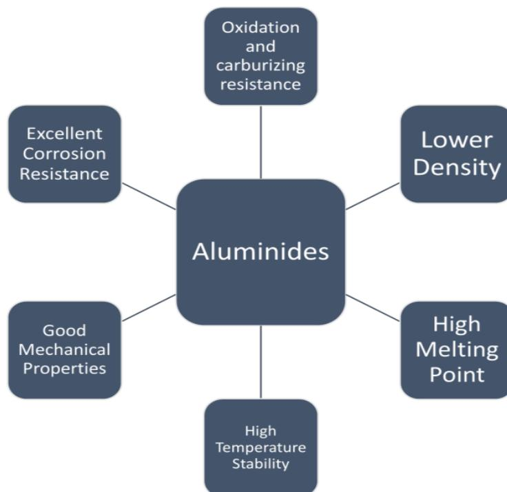
**Figure 4.** Characteristics features of Aluminides [12–15].
