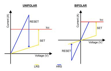
Figure 1. Unipolar and bipolar modes for RRAM devices.
