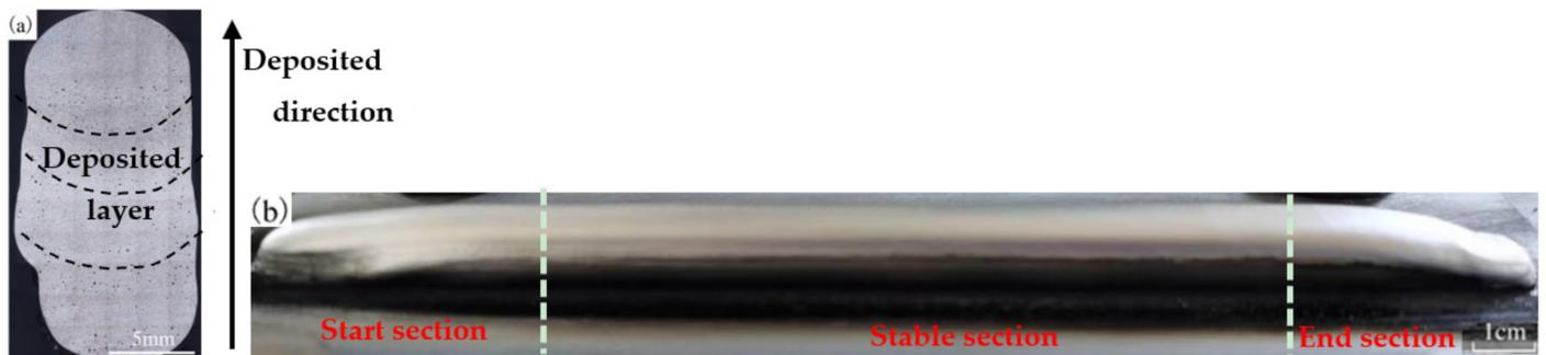
Figure 5. Cross section and morphology of deposited layer. (a) Deposition characteristics of deposited layer in the stable section of arc additive manufacturing. (b) Appearance morphology of forming characteristics of arc deposited layer.
