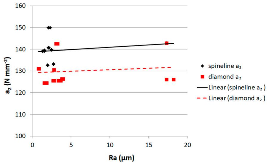
Figure 5. The relationship between Ra and parameter a<sub>2</sub>.
