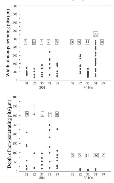
Figure 6. Non-penetrating pit depth and width of 304 and 304Cu after immersion in 6 wt.% FeCl<sub>3</sub> for 72 h.
