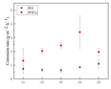
Figure 8. Corrosion rate from weight-loss measurements after a 72 h FeCl<sub>3</sub> immersion test.
