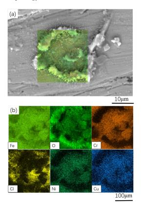
**Figure 1.** (a) SEM and (b) EDS mapping results of 304Cu pits after a 480 h salt spray test in 5 wt.% NaCl at  $35 \pm 2$  °C.
