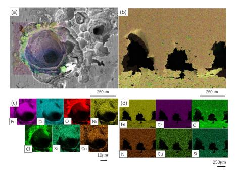
**Figure 5.** SEM morphology and EDS mapping results of 304Cu (**a**,**c**) non-penetrating and (**b**,**d**) penetrating pits after 72 h FeCl<sub>3</sub> immersion tests.
