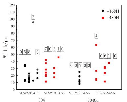
The pits were usually smaller than 50  $\mu$ m in width. However, there were large pits in the S1 sample of 304Cu, the size of which were more than 60  $\mu$ m.
