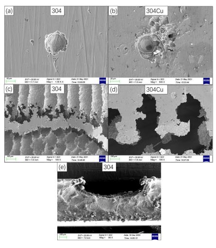
**Figure 4.** Morphology of (**a**,**b**) non-penetrating and (**c**,**d**) penetrating pits in 304 and 304Cu; (**e**) cross-section of 304 pits after 72 h FeCl<sub>3</sub> immersion tests.
