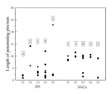
Figure 7. Length of penetrating pits on 304 and 304Cu after immersion in 6 wt.% FeCl<sub>3</sub> for 72 h.
