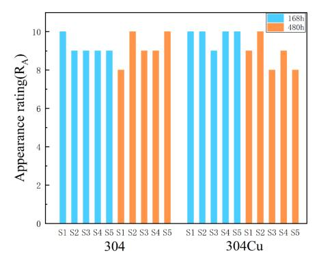
Figure 3. Appearance rating of stainless steel after salt spray test in 5 wt.% NaCl.
