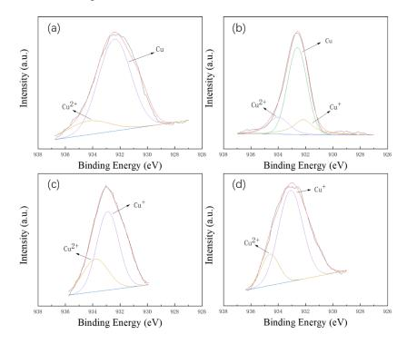
**Figure 9.** X-ray photoelectron spectroscopy analyses on Cu of (**a**) as-received 304Cu, (**b**) 304Cu after 168 h salt spray tests, (**c**) 304Cu after 480 h salt spray tests and (**d**) 304Cu after 72 h FeCl<sub>3</sub> immersion tests.
