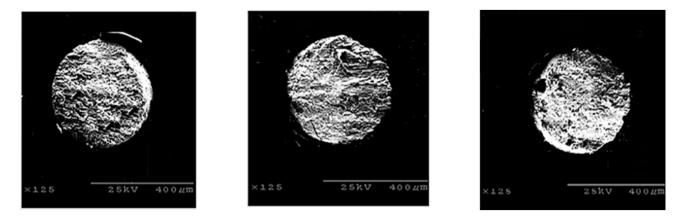
**Figure 34.** SEM images for tested joints under various dwelling periods compared with no dwelling condition (most left).
